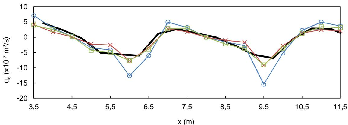
Figure 4. Measured data (thick black line) for  $d_{50}=0.465\text{mm}$ , test 30 (Schepers, 1978), revised grab and dump model (circles), with critical shear stress (squares) and traditional Meyer-Peter & Müller model (crosses)
