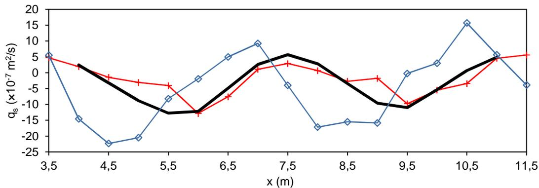
Figure 3. Measured data (thick black line), predicted sediment flux using percentages from Hallermeier (squares) and Migniot (crosses).
