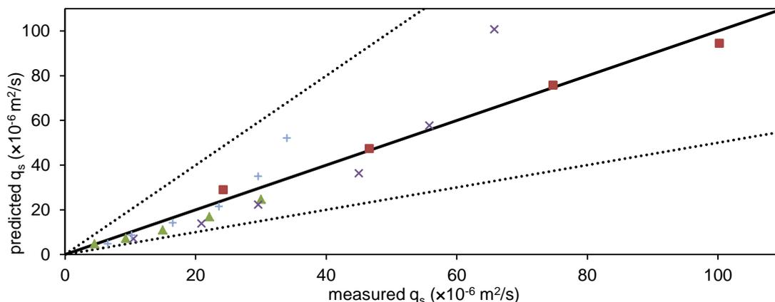
Figure 6. Model performance for revised grab and dump model under sheet flow conditions from van der A et al. (2010a) for  $d_{50}=0.15\text{mm}$ ,  $T= 5\text{s}$  (triangles),  $6\text{s}$  (squares),  $7\text{s}$ ( $\times$ ), and  $9\text{s}$ ( $+$ ). Solid line denotes 1:1 line, dotted lines are for a factor of 2 difference.
