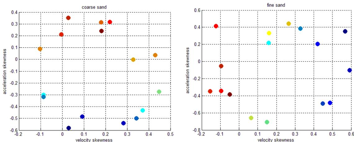
Figure 2. Velocity skewness and acceleration skewness for tests 30 and 6 with  $d_{50}=0.465\text{mm}$  and  $d_{50}=0.125\text{mm}$  respectively;  $q_s$  ranges from most positive (dark red) to most negative (dark blue). Data from Schepers (1978).
