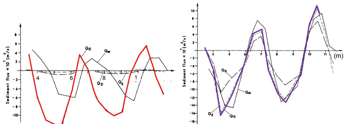
Figure 1. Predicted sediment flux from grab and dump model (bolded) for  $d_{50}=0.465$ mm (left) and  $d_{50}=0.125$ mm (right) from Nielsen (1988).  $Q_M$  is the measured sediment flux and the x-axis is the measurement from the wave maker (in metres).
