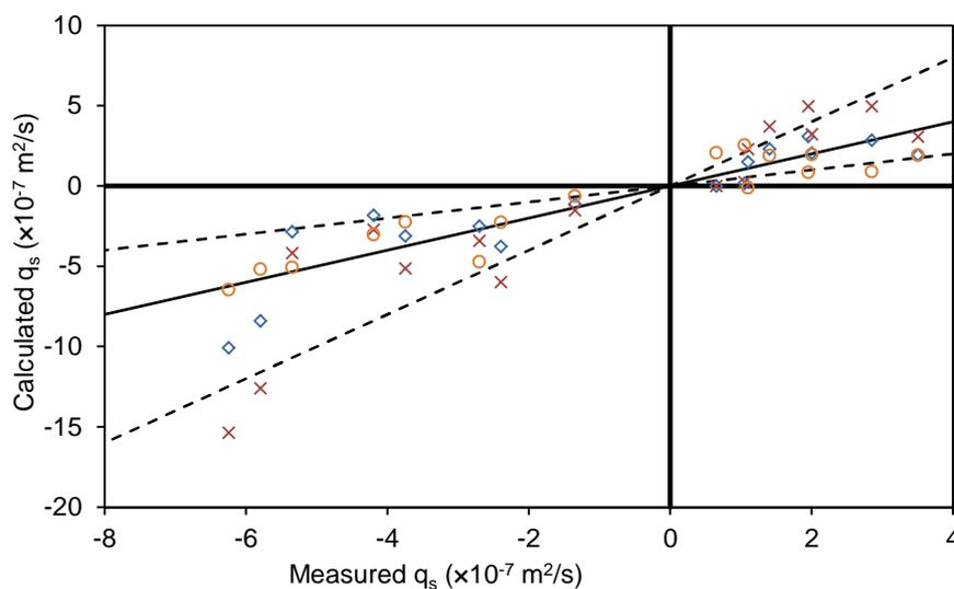
Figure 5. Model performance for revised grab and dump model (crosses), revised grab and dump model with critical shear stress (diamonds), and van der A et al.'s (2010b) model (circles) for test 30 from Schepers (1978). The solid line indicates 1:1 line, and the dotted lines show the lines for a factor 2 difference.
