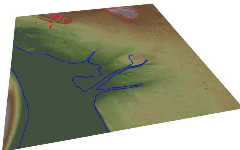
Figure 1. Digital terrain model of a Wadden Sea area generated from lidar data. Water covered tidal channels are outlined in blue, mussel beds in red.
