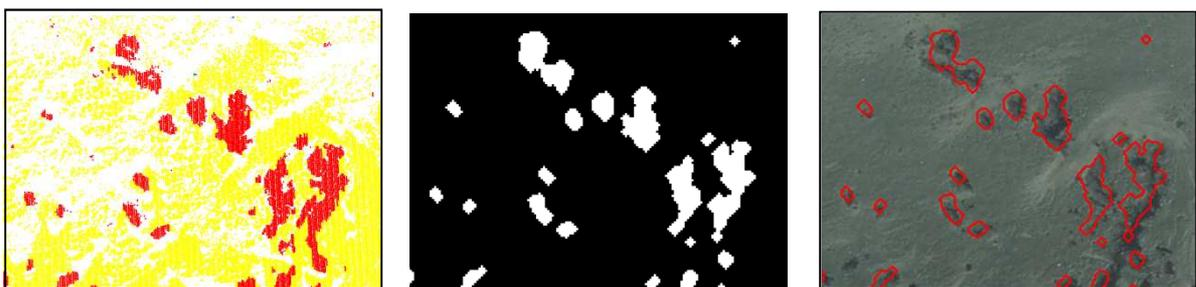
Figure 3. The labeled point cloud (left) is projected to a binary image (middle) of which mussel bed objects are generated and compared with an orthoimage (right).
