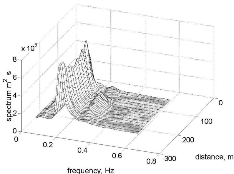
Figure 1. Spatial evolution of spectrum of irregular waves, showing a periodic energy exchange between first and second harmonics. Significant wave height at distance 230 m from the shore is 1.21 m. Wave spectra are normalized to the corresponding dispersions of wave ordinates. Wave data set No 39, registered on 29.09.2007 during field experiment “Shkorpilovtsy–2007”
