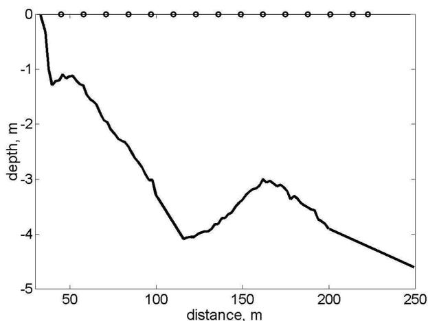
Figure 2. Bottom profile and location of wave gauges during the field experiment "Shkorpilovtsi-2007".
