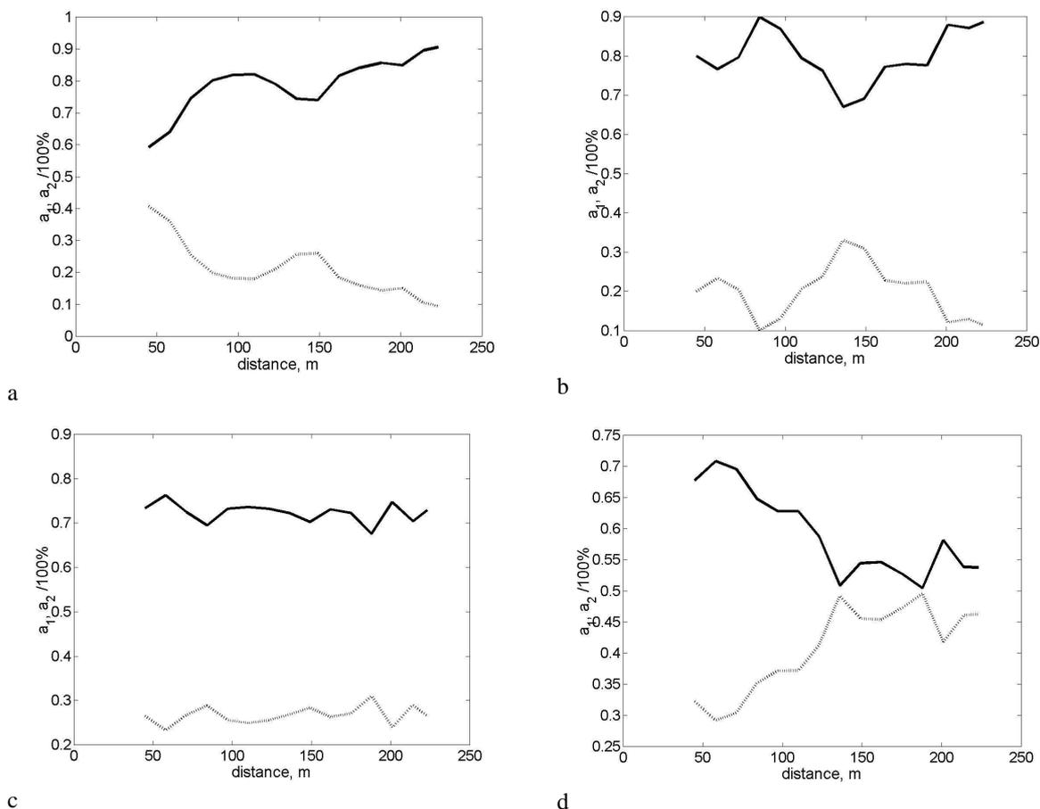
Figure 3. Scenarios of evolution of first and second harmonics in the coastal zone. Field experiment "Shkorpilovtsi–2007"; thick line - first harmonic amplitude ( $a_1$ ), dotted line - second harmonic amplitude ( $a_2$ ).
