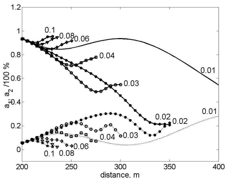
Figure 7. Evolution of energy of first and second harmonics during transformation of waves with JONSWAP spectrum and initial  $H_s = 1$  m,  $T_p = 7$  s,  $\gamma = 6$ , propagating over different bottom slopes; thick line - first harmonic amplitude ( $a_1$ ), dotted line - second harmonic amplitude ( $a_2$ ).
