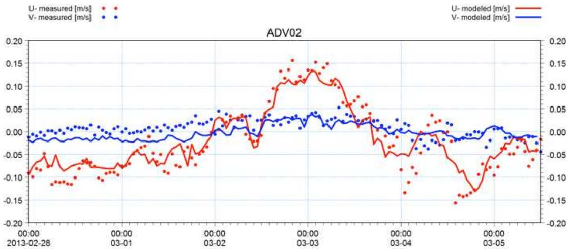
Figure 7. Model validation. Measured vs. Modeled currents in the onshore ADV location.
