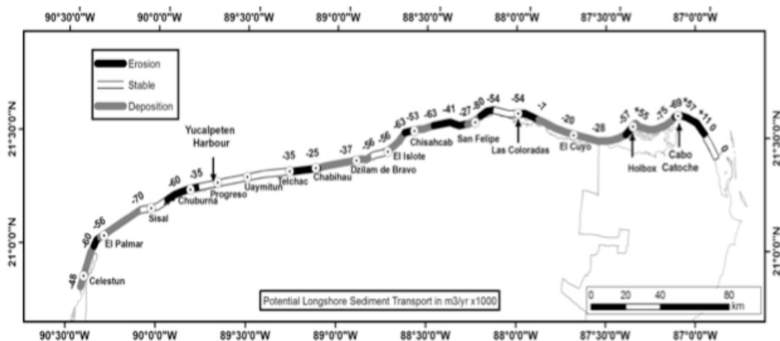
Figure 2. Potential erosive, depositional and stable sections of the northern Yucatan coast (adapted from Appendini et al., 2012).
