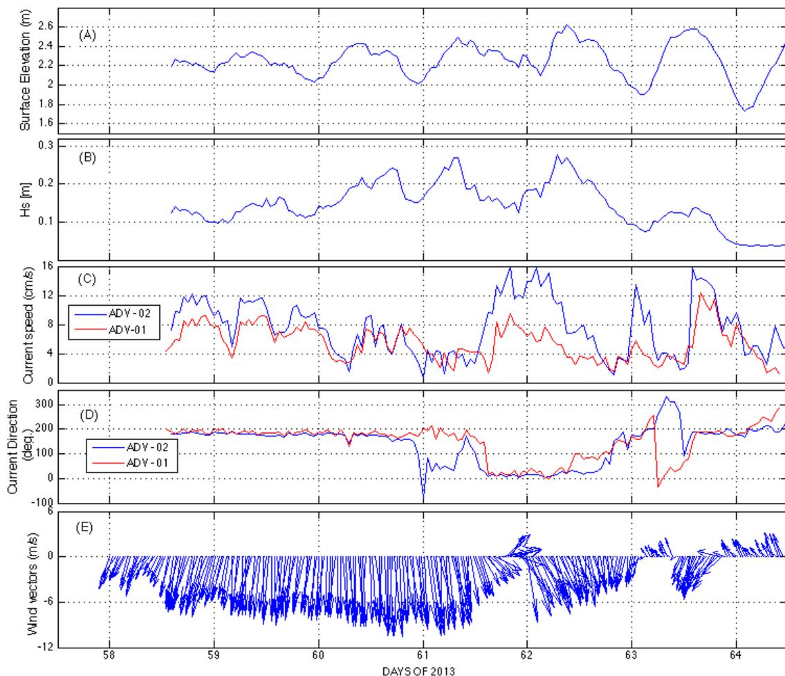
Figure 6. Wind and currents data from the ADV (offshore, ADV1, and onshore, ADV2, of the dune field): surface water level (panel A), significant wave height (panel B), both from the ADV-02, current speed from both ADV (panel C), corresponding current direction (panel D), and wind vectors (panel E).
