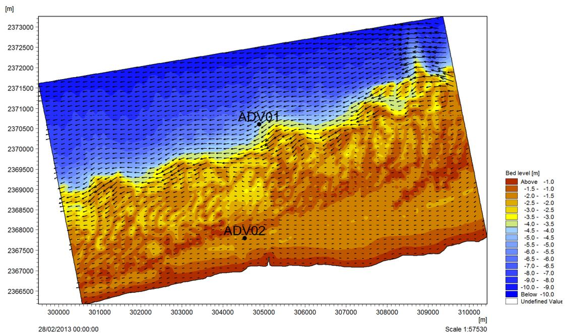
Figure 8. Initial bathymetry used to run the models.
