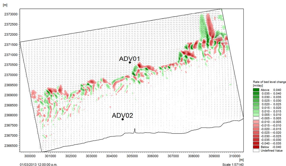
Figure 9. Simulated rate of bed level change.
