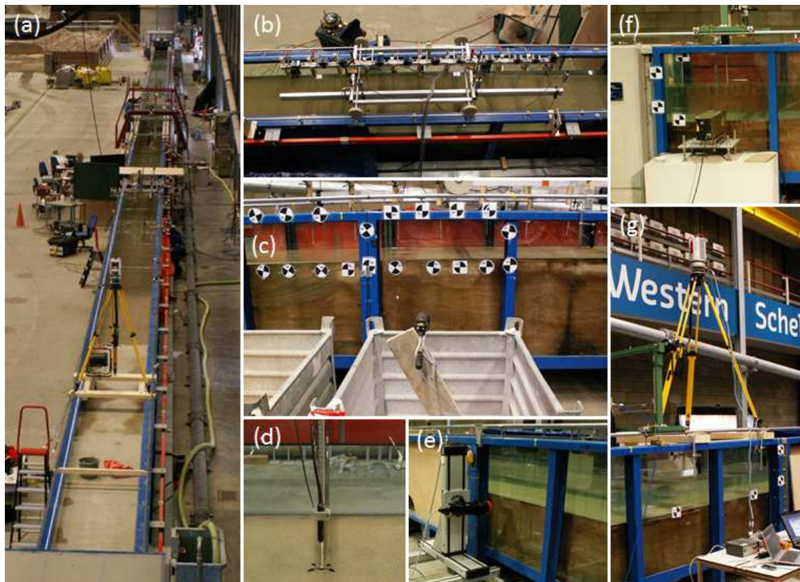
Figure 2. Photos showing the flume and various instruments deployed during GLOBEX. (a) Overview of the 110-m long flume in down-wave direction. (b) Trolley, instrumented with 11 wave gauges and 3 electromagnetic current meters; (c) Side-looking camera. (d) Acoustic Doppler velocimeter deployed in the swash zone; (e) Part of the Dantec LDA optics and traverse system; (f) Deltares LDV system; (g) Riegl VZ-400 Terrestrial Laser Scanner. All photos except (d) taken by B.G. Ruessink; photo (d) by Dominic van der A.
