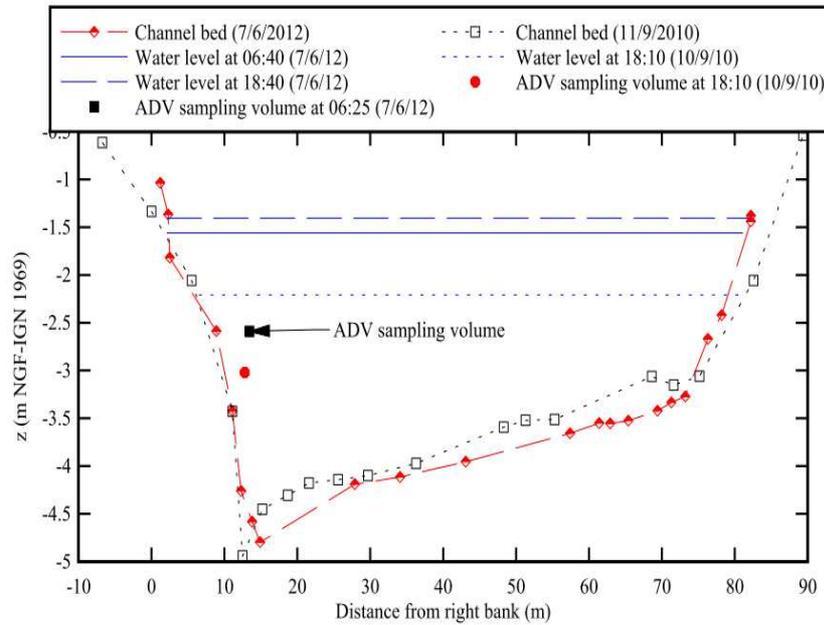
Figure 3. Surveyed (distorted) cross-section looking upstream - Comparison between the 2010 and 2012 surveys at the same cross-section
