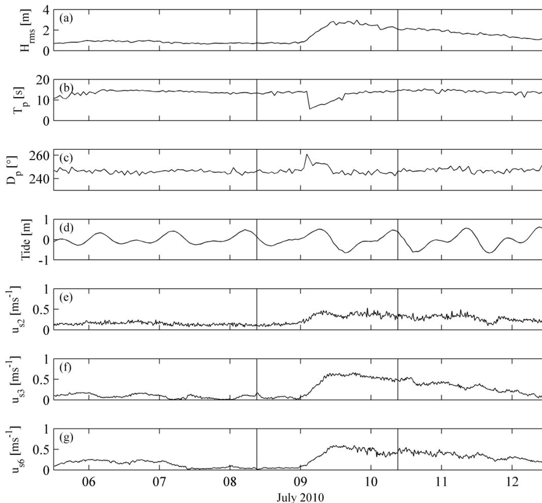
Figure 2. Hydrodynamic measurements obtained in the field experiment. The vertical lines denote the period considered in the numerical model component of this study. (a) Root Mean Squared wave height, (b) peak wave period, (c) peak wave direction and (d) tidal elevation measured on the forereef at S1. (e-g) Depth averaged velocity magnitude for the three sites in the reef (S2, S3, S6), respectively.
