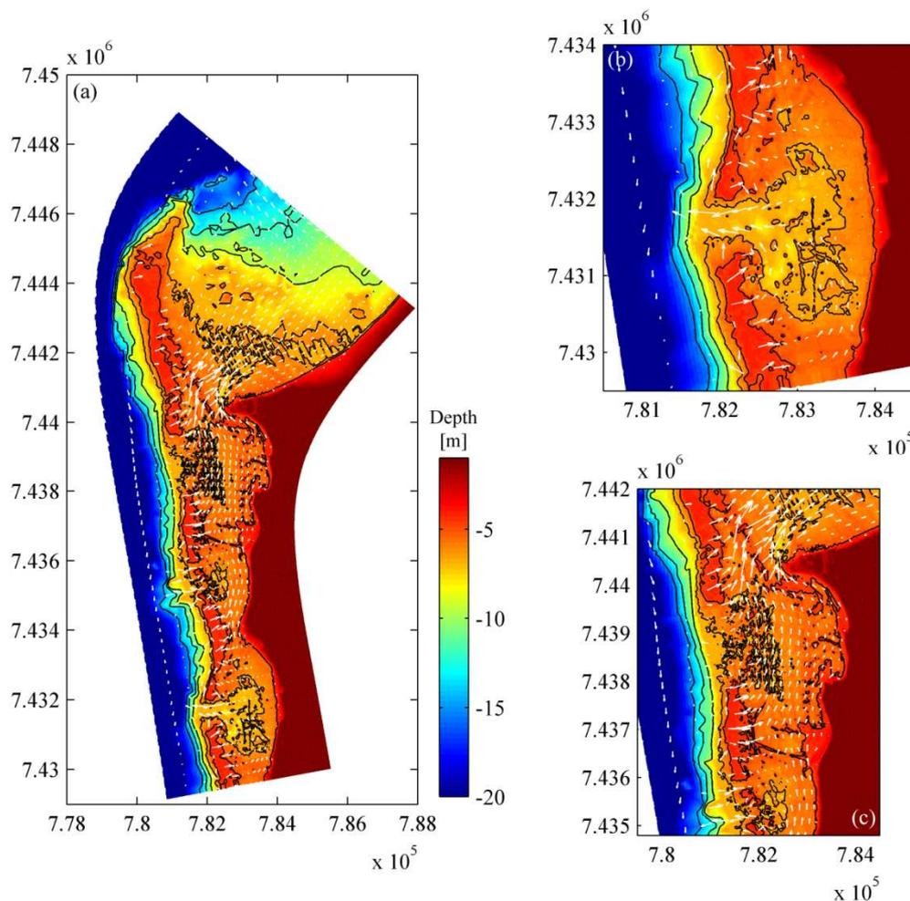
Figure 4. (a) Eulerian current velocity vectors for the whole domain (b) Higher resolution velocities for the southern half of the domain (c) Higher resolution velocities for the northern half of the domain. The vectors displayed in each figure have been plotted on a 10 m x 10 m vector scale.
