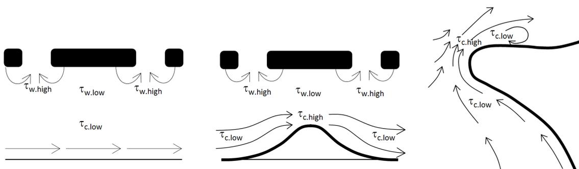
Figure 6. Conceptual feature development. (a) Dominant processes that result in the development of a cusped foreland (b) Change in bed shear stresses due to the development of the cusped foreland (c) Development of Point Maud by accelerated flow and a depositional eddy.
