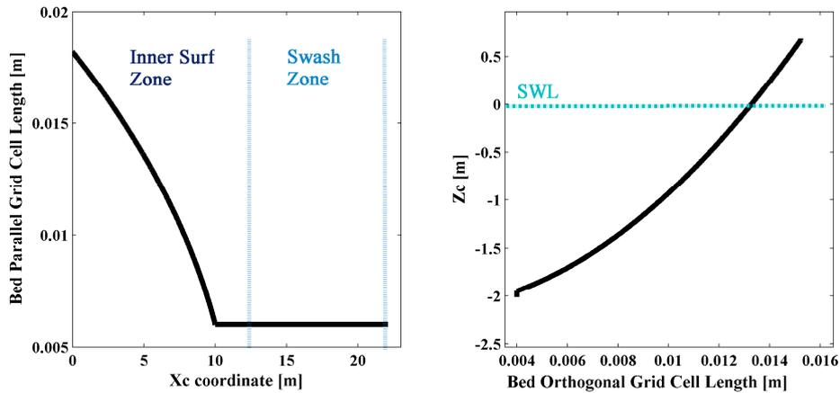
Figure 2. Horizontal (left) and vertical (right) non-uniform grid variation within the computational domain.
