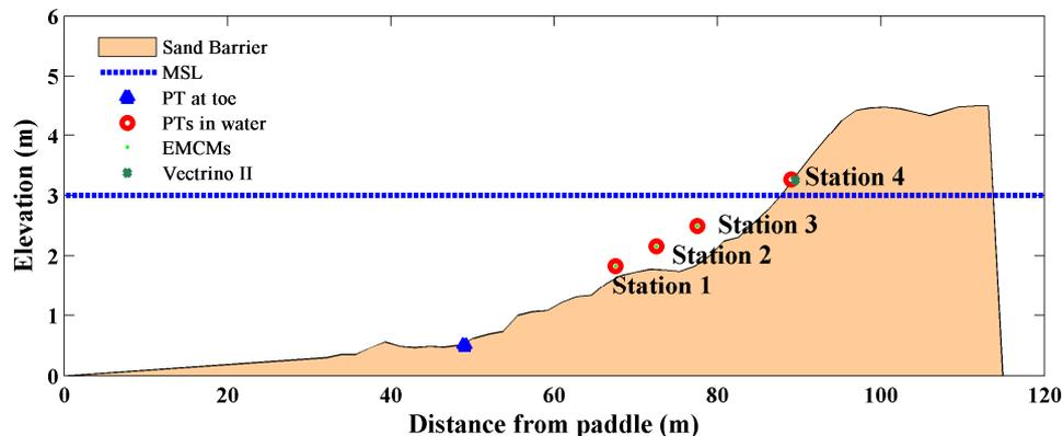
Figure 1. BARDEX II experimental setup and computation domain. The reference frame in the numerical model is oriented bed parallel and bed orthogonal to bed. Numerical results from a coarse mesh resolution (*black dash square*) were employed for the forcing of a fine mesh (*red dashed square*) in order to resolve boundary layer processes within the swash zone.
