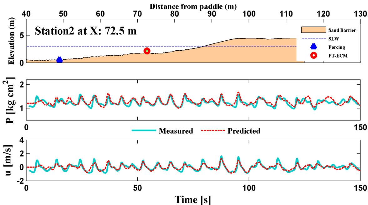
Figure 5. Measured (in light blue) and predicted (in dashed red) bottom pressure and velocity time series at Station 2.
