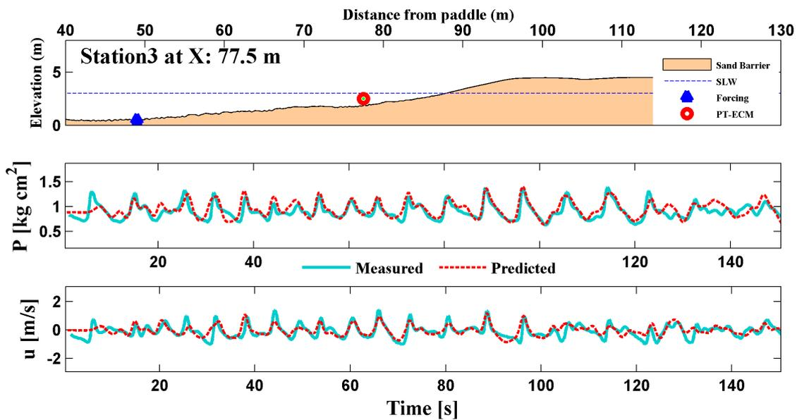
Figure 6. Measured (light-blue) and predicted (dashed-red) mid water pressure and velocity time series at Station 3.
