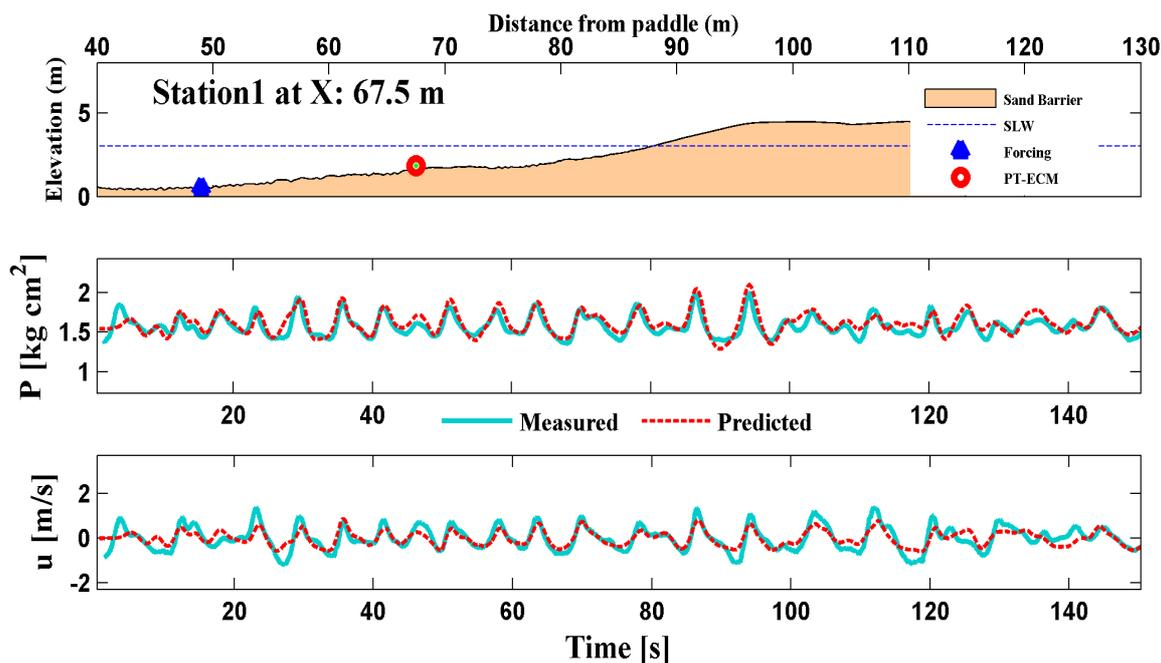
Figure 4. Measured (light blue) and predicted (dashed-red) bottom pressure and velocity time series at Station 1.
