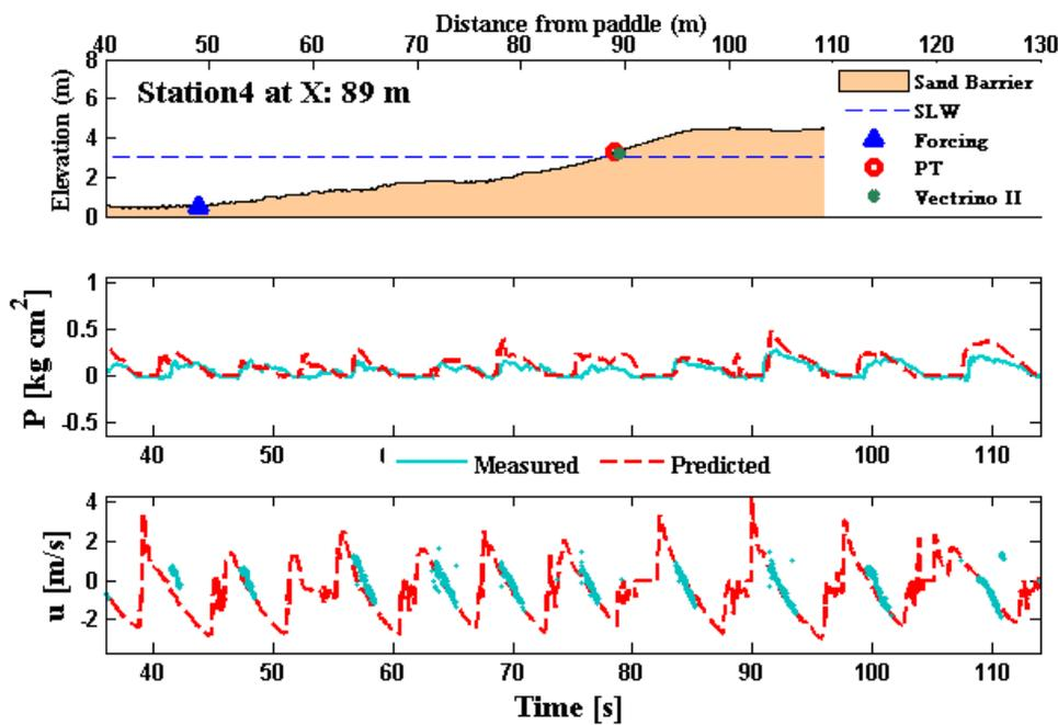
Figure 8. Dynamic pressure and velocity time series at station 4 (measured: *light blue*; predicted: *dashed red*).
