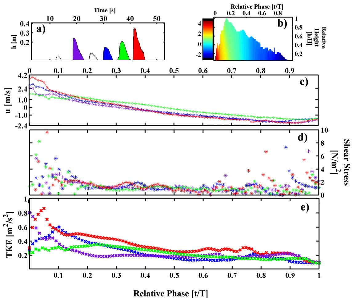
Figure 12. (a) Varying water depth evolution at  $x=91.5$  m. (b) Time and height normalization of swash event depicted as red in a). The color bar indicates cross-shore velocity [m/s] at 0.002m above the bed. (c) Horizontal velocities; (d) Bed shear stresses and (e) turbulent kinetic energy of predicted swash events.
