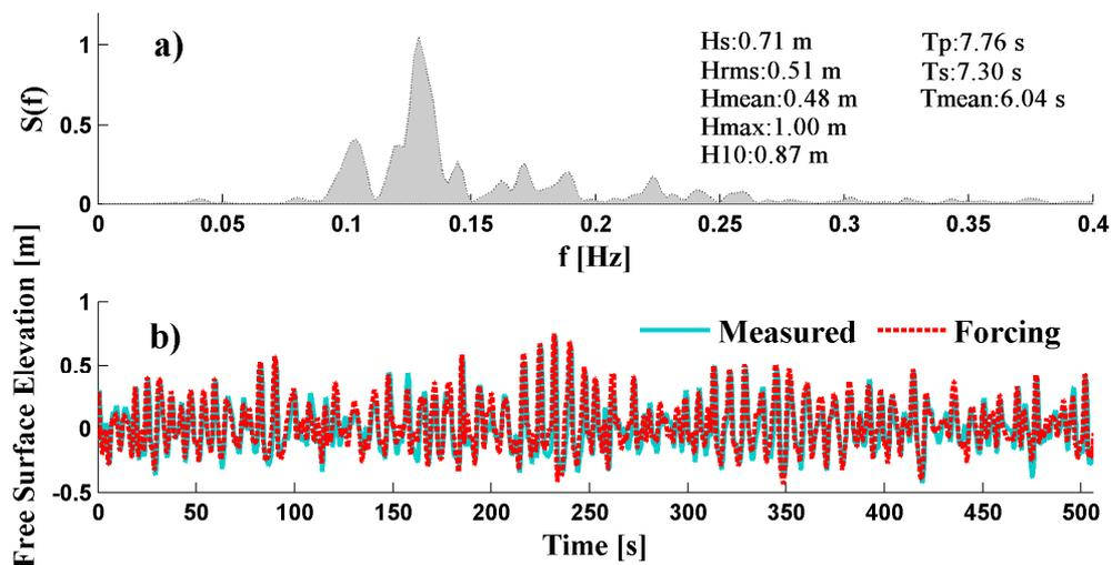
Figure 3. (a) Spectral characteristics employed as the forcing wave signal. (b) Measured and simulated time series at the forcing boundary.
