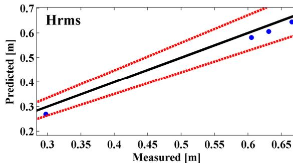
Figure 7. Measured versus predicted root mean square wave height for all stations. Solid line: perfect agreement; dashed red line:  $\pm 10\%$  confidence interval bounds.
