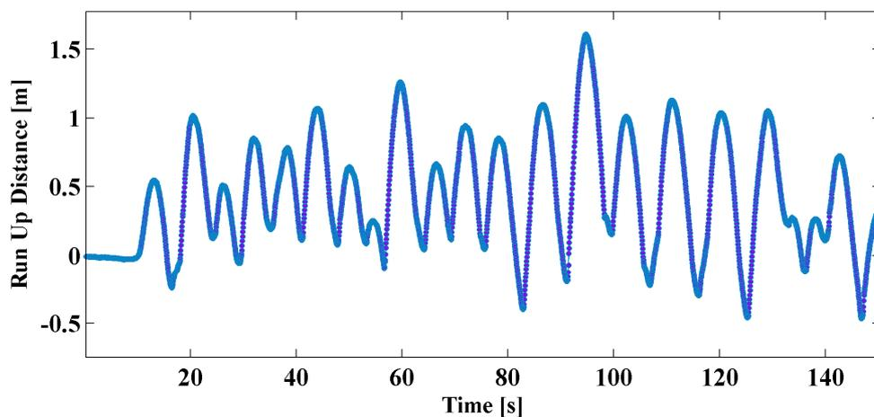
Figure 11. Predicted time series of run up distance evolution from still water (x=87.5 m).
