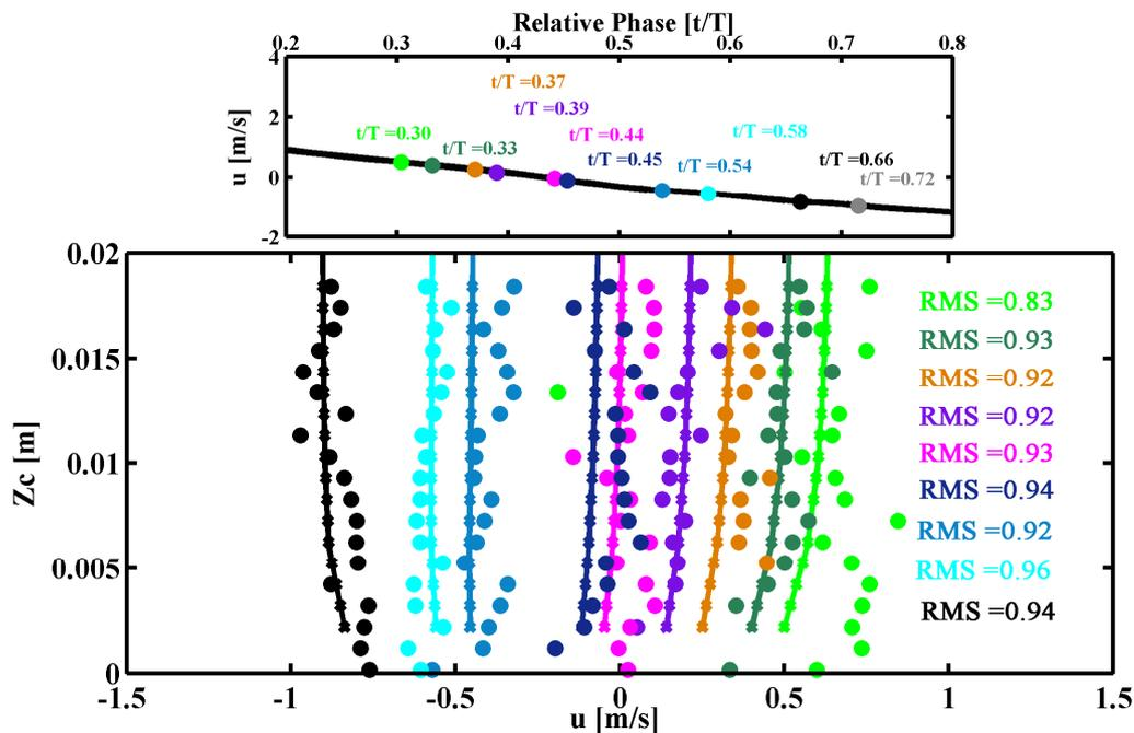
Figure 10. Measured (colored filled circles) and predicted (colored crossed lines) horizontal velocity profile for a swash event from bed until 0.02m above bed and corresponding root mean square error (RMS) obtained values.
