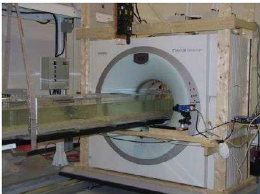
Figure 1. CT-scanner with the flume passed in the gantry and PIV (structure is now in aluminium instead of wood)
