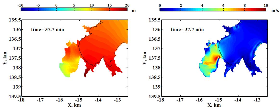
Figure 7. Left: Calculation result of water surface elevation at the uprush phase of the first tsunami. The time counts for the elapsed time from the occurrence of earthquake. It is found that the tsunami overflowed from the whole stretch of Nehama Beach. Right: Magnitude of velocity at the same phase. Flow velocity at the south end of Nehama Beach was so large that sediment deposited there was supposed to be transported inland.
