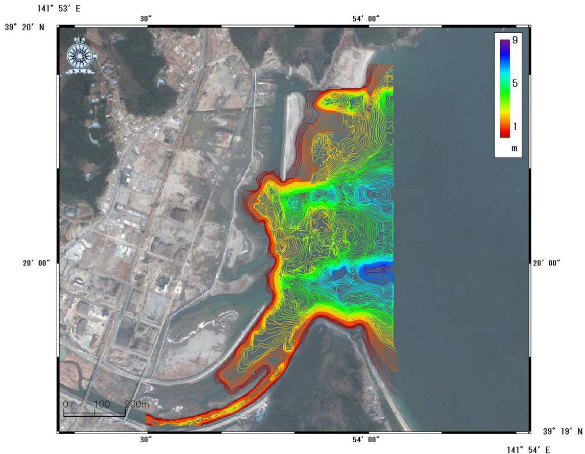
Figure 6. Bathymetry data obtained by depth measurement in June 2012. It is clearly seen that a few deep trenches were created further along the old river channels. It is found from the bathymetry that the sandbar was completely washed away.
