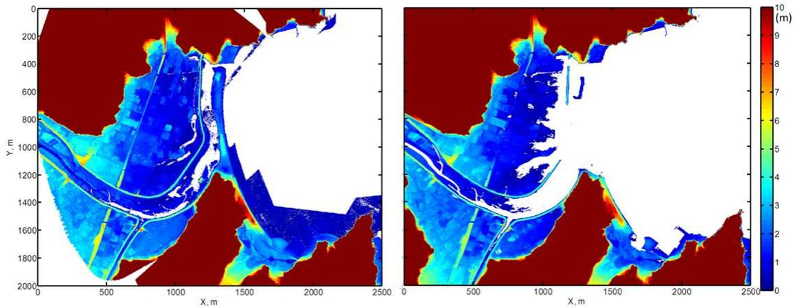
Figure 4. 2 m by 2 m resolution Laser-Profiler (LP) data of ground level provided by the Ministry of Land, Infrastructure, Transport and Tourism, Japan for topography before 2011 Tohoku Tsunami (Left) and after (Right). The water area is left blank (or recorded as 0 m for altitude).
