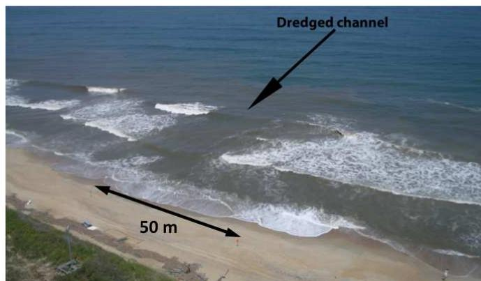
Figure 2. Normally incident waves breaking (white foam) on the shallow sides of the deeper dredged channel (arrow).
