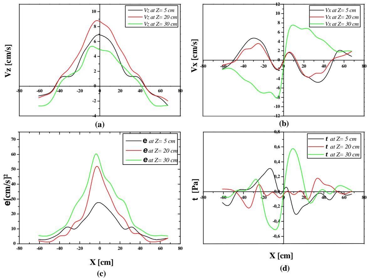
Figure10. The horizontal profiles at three positions ( $Z = 5\text{cm}, Z = 20\text{cm}$  and  $Z = 35\text{cm}$  from the bottom) : a) the vertical velocity  $V_z(x)$ ; b) horizontal velocity  $V_x(x)$ ; c) kinetic energy  $e(x)$ ; d) the shear rate  $\tau_{xz}(x)$
