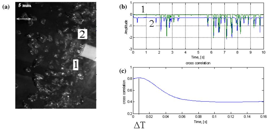
Figure 2: a) photograph of the double-tip conductivity probe. b) double-tip conductivity probe outputs. c) cross-correlation function for a dual-tip probe
