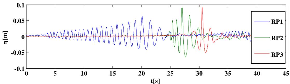
Figure 5. Evolution of wave packet along the channel. Time series of free surface displacement  $\eta$  are recorded by three transducers for a pulse with averaged frequency  $f=0.75 \text{ Hz}$ .
