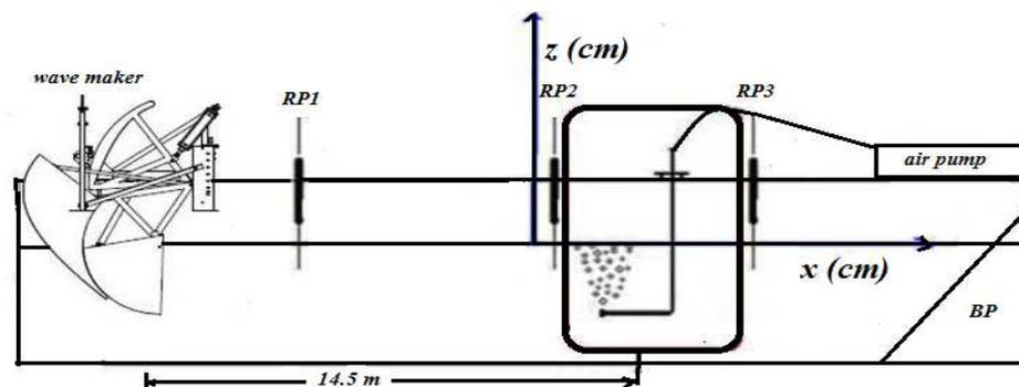
Figure 1. Experimental setup: RP1, RP2, RP3 are resistive probes free surface measurement, PB is porous beach.
