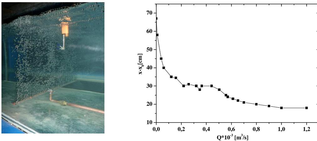
Figure 3 a) photograph of air bubbles curtain. b) Dependence of wave breaking coordinate ( $X-X_0$ ) on flux  $Q$
