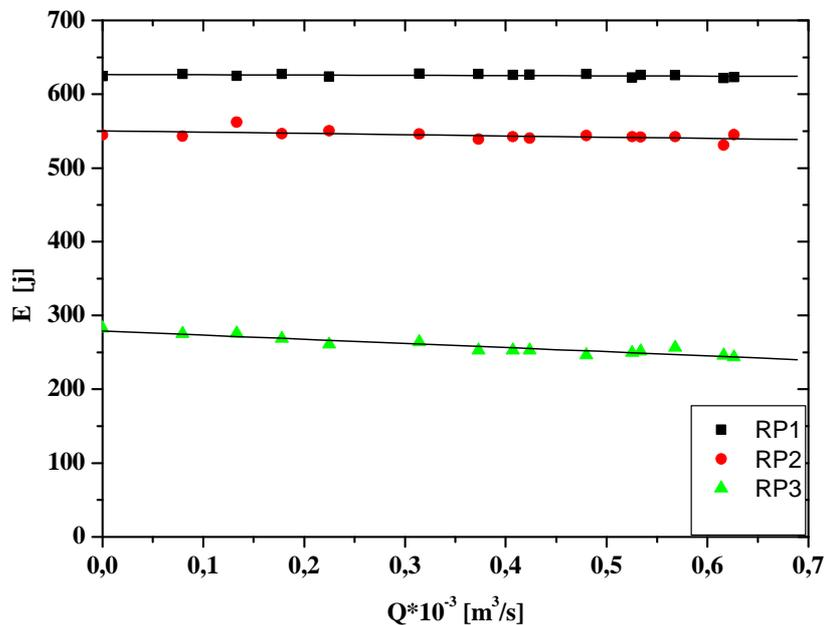
Figure 6. Dependence of wave packet energy on air flux; probes PR1,2 are situated in the flume before wave breaking point, PB3 is behind this point. .
