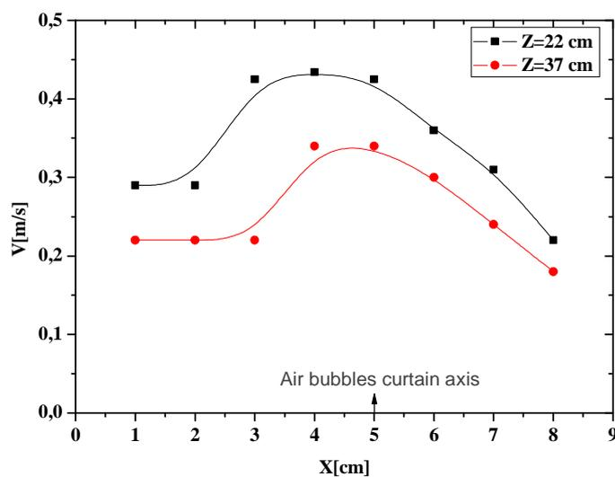
Figure 8. Horizontal profile of vertical velocity of bubbles for two depths (air flux  $Q = 1.2 \cdot 10^{-3} \text{ m}^3/\text{s}$ ).
