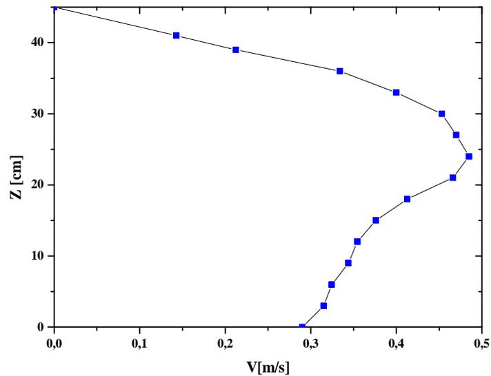
Figure 7. Vertical velocity of bubbles versus vertical coordinate z for an air flux  $Q = 1.2 \cdot 10^{-3} \text{ m}^3/\text{s}$ .
