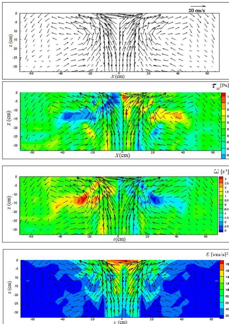
Figure 9. Fields generated by air bubble curtain, air flux  $Q = 1.2 \cdot 10^{-3} \text{ m}^3/\text{s}$ : a) velocity fields, b) vorticity fields, c) shear rate fields, d) kinetic energy fields.
