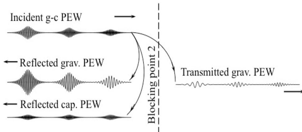
Figure 6. Mode conversion in the case of gravity-capillary waves at the blocking point 2 for the PEWs only.
