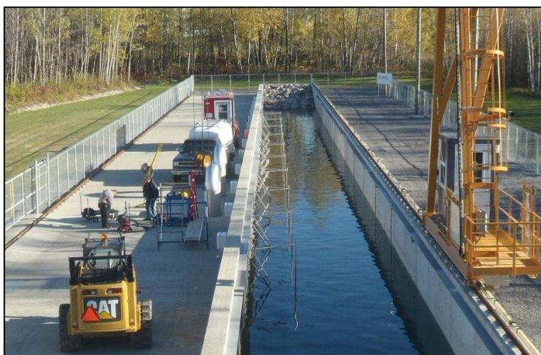
Figure 2. View of the monitoring stations. They are located along the left wall of the flume with a spacing of 5 m and they delimit a test section of 65 m long (photo credit: Corinne Brunelle).
