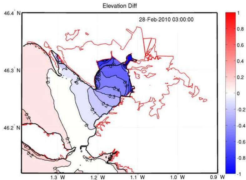
Figure 8. Difference between a simulation performed with a grid enabling flooding and a simulation without flooding, suggesting much lower water levels in the flooding case.
