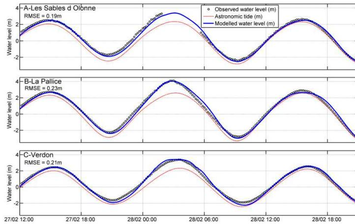
Figure 4. Validation of elevation and storm surge in La Pallice with ARPEGE wind ( black circle: observed water level, red line: astronomic tide, blue line: modelled water level, )
