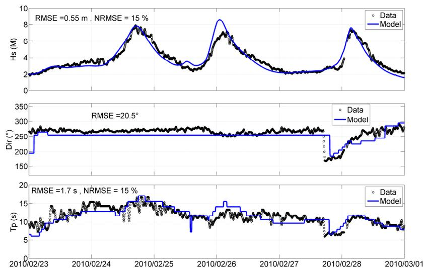
Figure 3. Validation of wave result at the Datawell Buoy offshore Oléron Island (figure 1) for Significant wave height and peak direction and period (blue dots: observed data, green line: model result).
