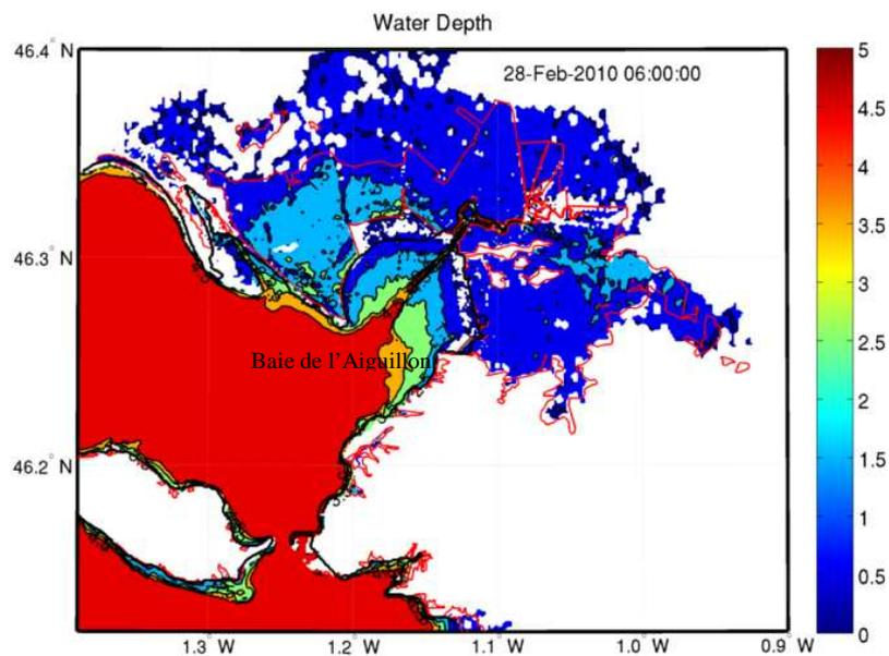
Figure 5. Maximum water depth simulated during Xynthia showing the extent of the simulated flooding compared to the observed one (red line).
