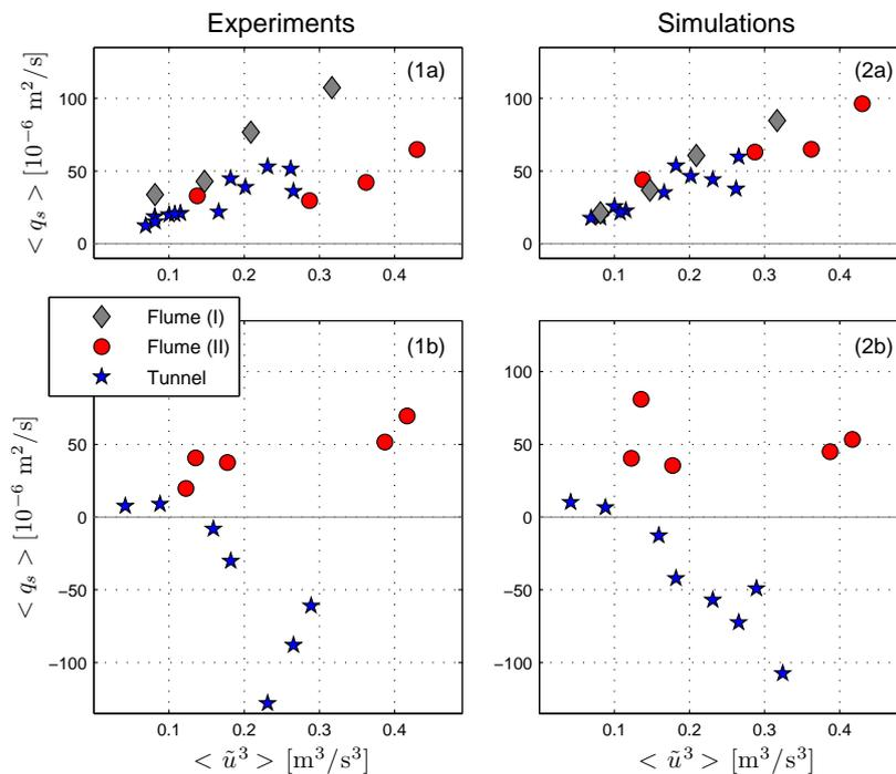
Figure 5. Measured (1a,b) and computed (2a,b) net sediment transport rates  $\langle q_s \rangle$  of medium (panels a) and fine (panels b) sands against the third order velocity moment determined from the oscillating part of the horizontal velocity  $\tilde{u}$ , for various experimental conditions from both tunnel and flume experiments.
