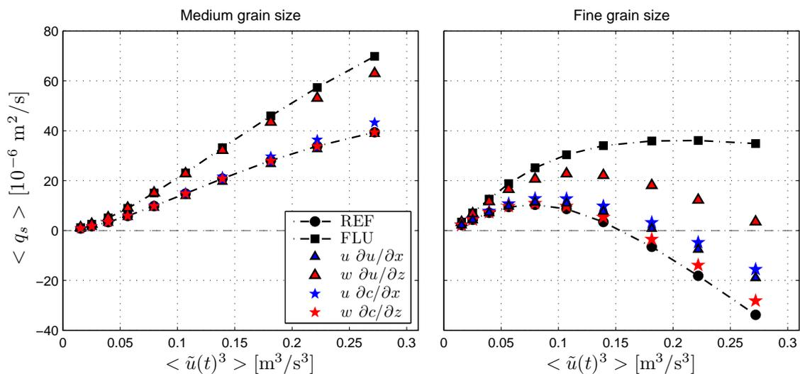
Figure 6. Net transport rates  $\langle q_s \rangle$  of medium (0.25mm) and fine (0.14mm) sized sediments for velocity skewed waves with increasing wave height, here plotted against  $\langle \tilde{u}^3 \rangle$ . The figure shows results obtained with all advective terms switched on (FLU), all advective terms switched off (REF), and only  $w\partial u/\partial z$ ,  $u\partial c/\partial x$  or  $u\partial u/\partial x$  switched on.
