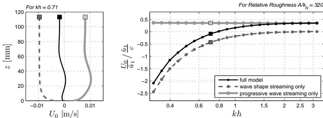
Figure 4. Streaming velocities from full model simulations (black), simulations with wave shape effect only (gray / dashed line), and progressive wave effect only (light gray); Left) streaming profiles for a single  $kh$ -value; right) non-dimensional streaming at the outer edge of the boundary layer as function of relative water depth  $kh$  (on log-scale) for  $A/k_N = 320$ .
