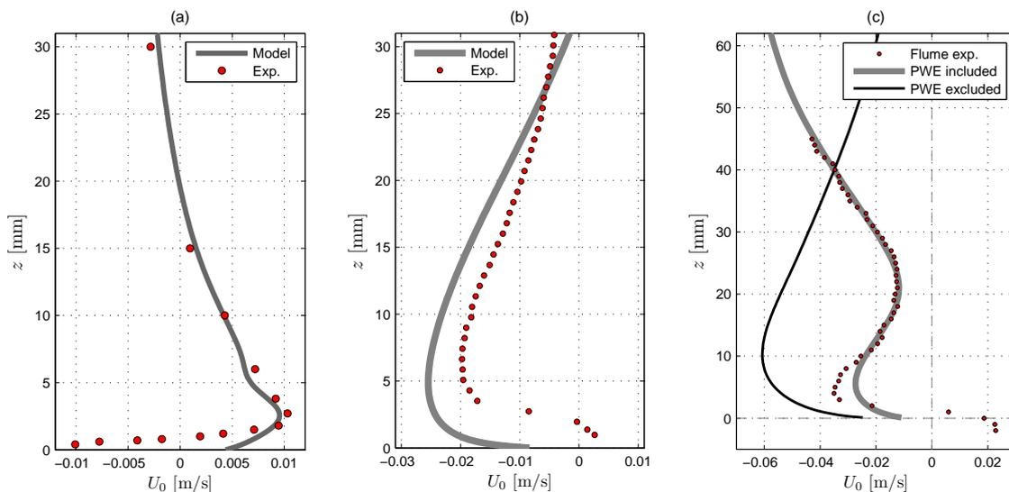
Figure 3. Model-data comparison on wave averaged velocity  $U_0$  for (a) a sine wave in a small scale flume experiment, (b) a velocity-skewed oscillatory flow in a tunnel experiment, (c) a velocity-skewed wave in a large scale flume experiment.
