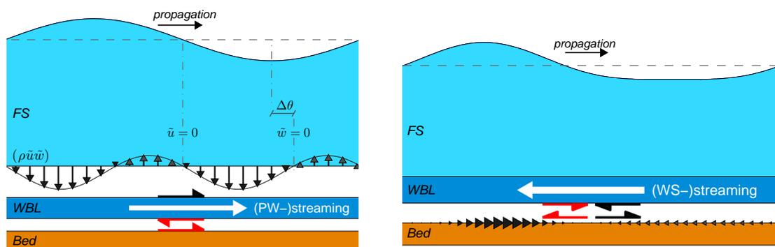
Figure 2. Schematic drawing of boundary layer streaming mechanisms; (a) Progressive Wave Streaming; (b) Wave Shape Streaming; Small black arrows: wave-generated momentum transport (a) or bed shear stress (b); Black shear arrows: resulting wave-averaged stress; White arrow: generated current; Red shear arrows: current-related bed shear stress.
