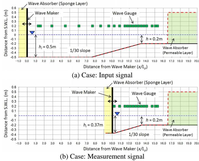
Figure 2. Numerical setup for bathymetry type 1.
