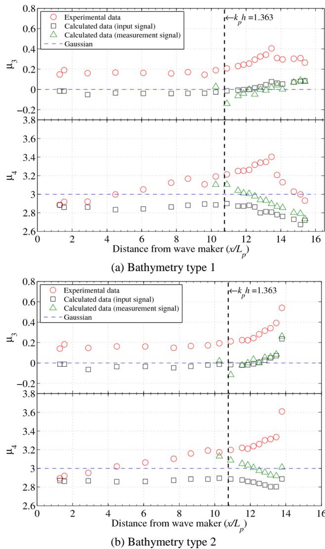
Figure 3. Spatial distributions of skewness and kurtosis simulated using the Boussinesq model for the bathymetry type 1 and 2. (circle: experimental data, square: simulated data for input signal, triangle: simulated data for measurement signal, shin dashed line: Gaussian distribution)
