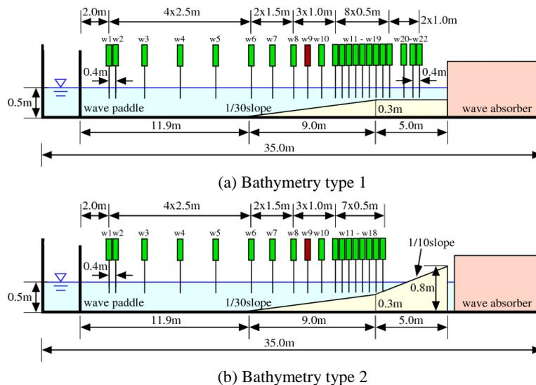
Figure 1. Cross sectional view of bathymetry configurations.
