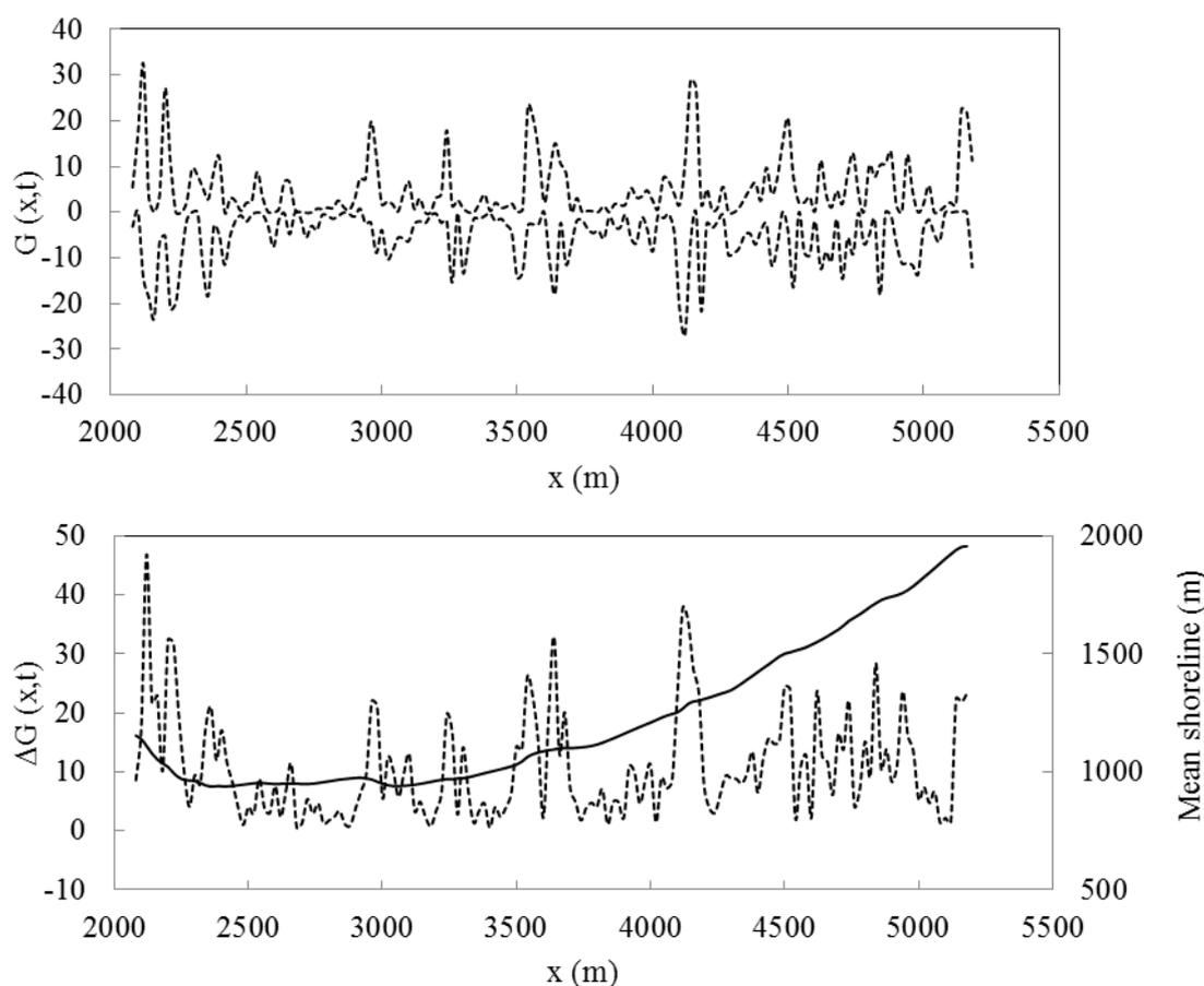
**Figure 5** – Envelope of the spatial variation of source function along the Colwyn Bay beach [top] Maximum variation of the source function at all longshore locations (dotted line) and mean shoreline position (dark line) [bottom].
