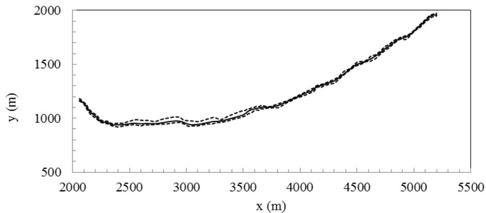
**Figure 3** – The mean shoreline and the shoreline envelope at Colwyn Bay during 2001 and 2005.
