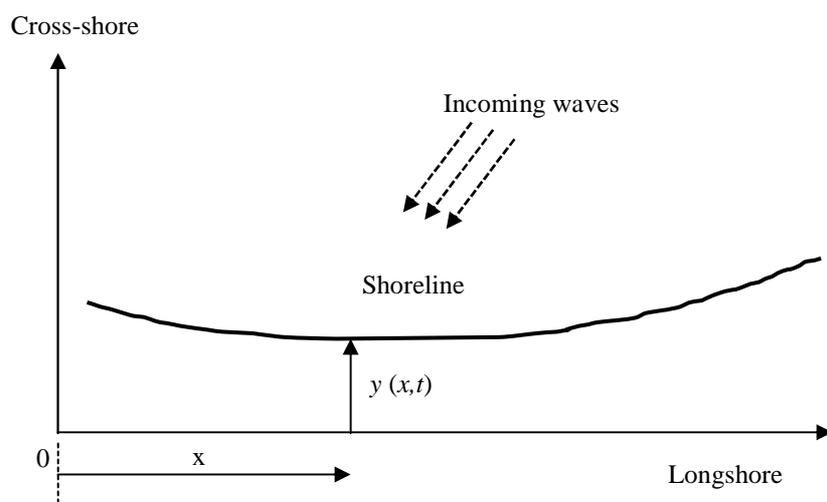
Figure 1 – Schematics of the beach plan shape model.
