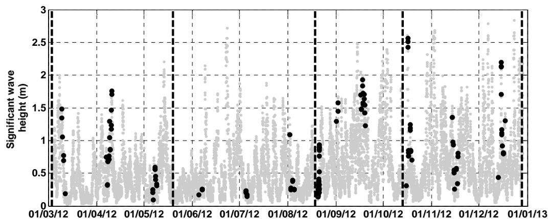
Figure 3. Significant wave height measured at Morecambe Bay buoy from 3<sup>rd</sup> March – 28<sup>th</sup> December 2012. The bold points show the events with the wave directions between 203-293  $^{\circ}$  (SSW and WNW) measured at water level above +5.0 OD.
