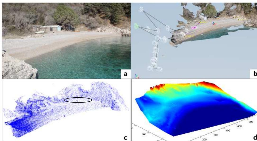
Figure 5. Reconstruction of a beach digital elevation model at Uboka cove: a) photo taken from one of the locations close to the beach; b) locations from which photos were taken; c) a point cloud derived by 123d Catch, the area which is 'static' is shown with black circle; d) digital elevation model obtained using a point cloud and geo-referencing transformation tools written in Matlab®.
