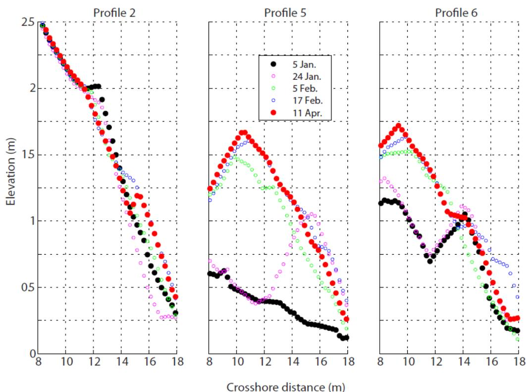
Figure 8: Beach profiles derived from digital elevations model at locations 2, 5 and 6 as given in Figure 6.
