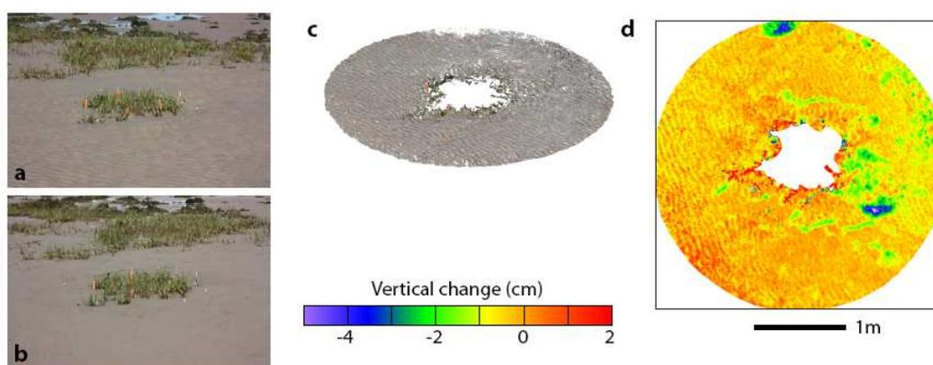
Figure 4. Digital elevation model of erosion and deposition around a *Spartina* tussock: a) photo taken on 20<sup>th</sup> June 2011; b) photo taken on 22<sup>nd</sup> June 2011; c) point cloud created for the image taken on 20<sup>th</sup> June 2011; d) difference map between 22<sup>nd</sup> and 20<sup>th</sup> June 2011.
