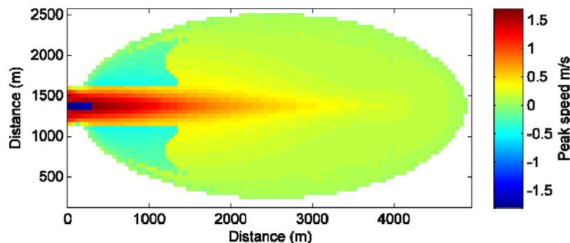
Figure 5. Peak velocity magnitudes from simulations with tide-forcing only. Negative (positive) values indicate that the peak velocity occurs during the ebb (flood) phase of the tide.
