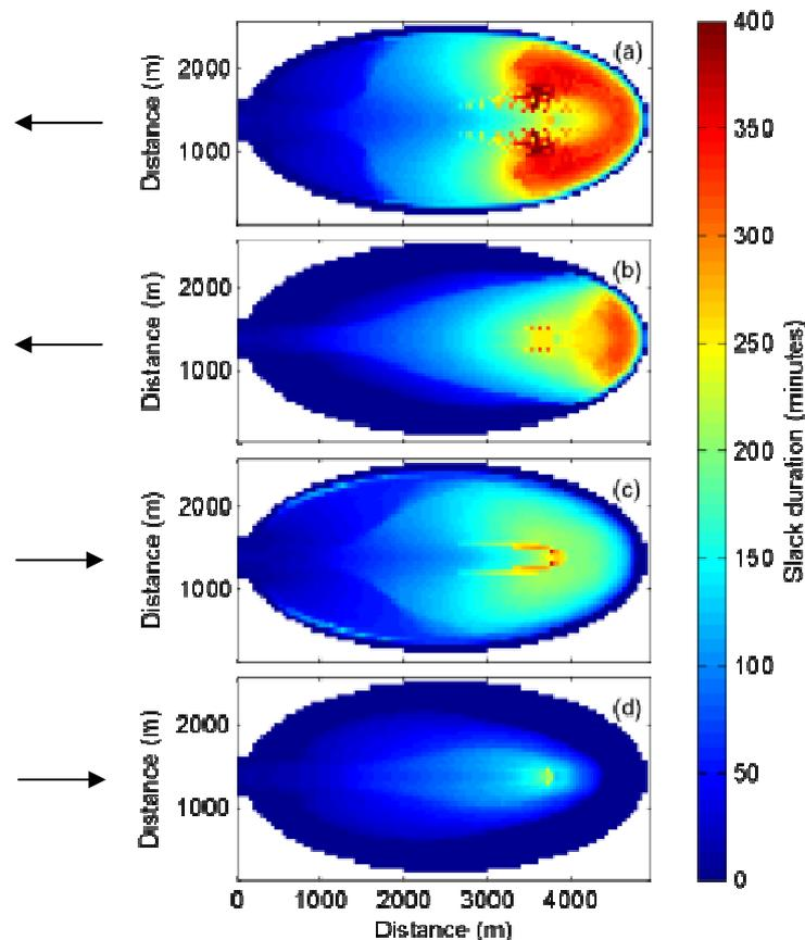
Figure 8. Slack duration as a result of combined maximum bed shear stress in minutes under a 5m/s (a) and 10m/s (b) seaward wind and a 5m/s (c) and 10m/s (d) landward wind. Wind direction is indicated with arrows.
