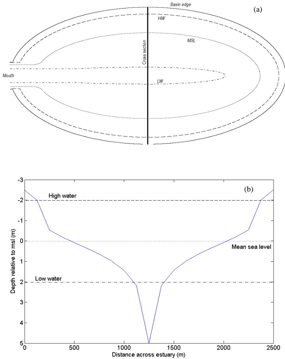
Figure 2. Schematic representation of the unfilled ( $\gamma=4.0$ ) estuary: (a) showing overhead view and (b) side view along the central North-South cross-section marked in (a). Low water, mean sea level and high water are shown to illustrate the intertidal form.
