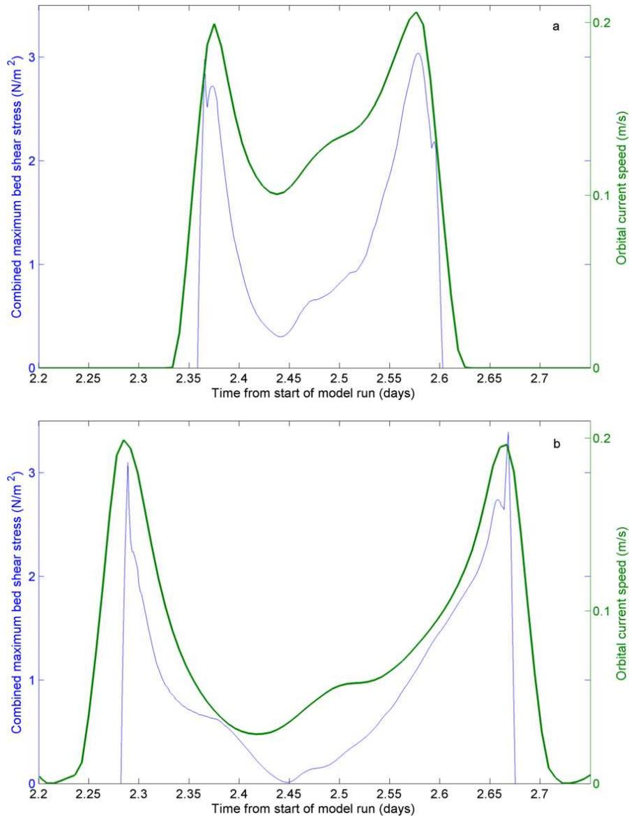
Figure 9. Wave orbital current speed (thick green line) and resultant bed shear stresses (thin blue line) shown for a shallow (a) and deep intertidal area (b).
