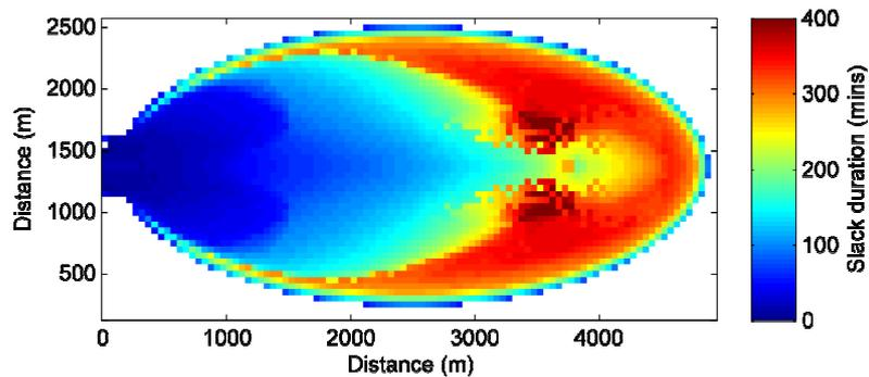
Figure 6. Slack water duration in minutes at high water defined as the amount of time that bed shear stress drops below the entrainment threshold for a sediment particle of 100 micron.
