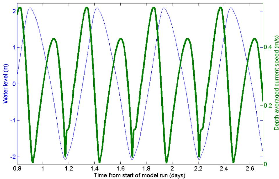
Figure 3. Example timeseries of water levels (thin blue line) and depth averaged velocities (thick green line) taken from the central subtidal area of the model.
