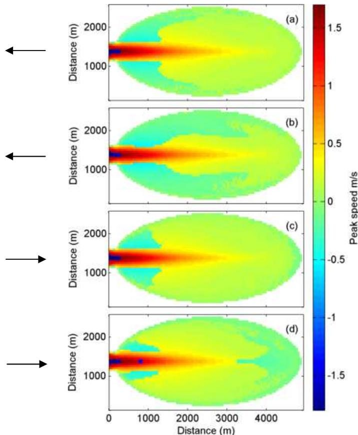
Figure 7. Peak velocity magnitudes for 5 (a) and 10m/s (b) seaward wind and 5 (c) and 10m/s (d) landward wind, negative (positive) values indicate that the peak velocity occurs during the ebb (flood) phase of the tide. Wind direction is indicated with arrows.
