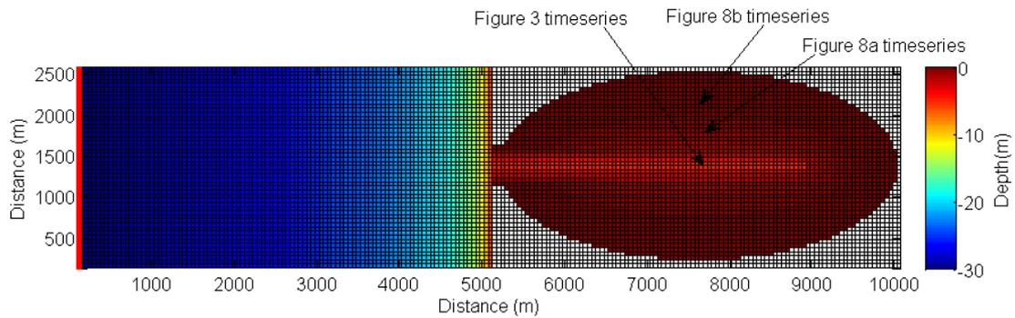
Figure 1. Numerical model grid and bathymetry. The model is forced at the single open boundary on the left hand side of the domain (thick red line). The locations from which the time series shown in Figures 3, 8a and 8b are indicated by the arrows.
