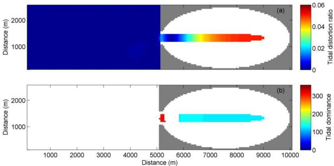
Figure 4. Plan view of distortion magnitude (a) (equation 3) and resultant direction of peak-velocity from distortion (b) (equation 4). Figure 4b only shows phase difference in subtidal areas where the distortion is significant ( $>0.01$ ). Simulations for an infilled mature estuary ( $\gamma = 4$ ) and tide only forcing. Grey areas denote land.
