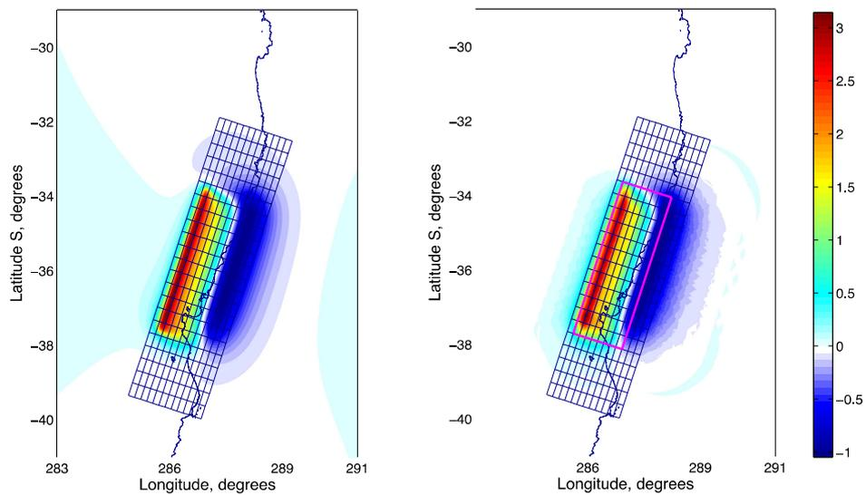
**Figure 3.** Reconstruction of the sea floor deformation combining linearly unit sources involved. Sea floor deformation of a probable scenario using Okada model (left panel). Reconstructed sea floor deformation by a linear combination of unit sources within pink rectangle (right panel). Colormap is vertical displacement in meters.
