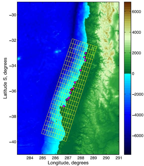
**Figure 2.** Mw7.0 unit sources covering the rupture zone of the 2010 Chilean Earthquake (yellow grid). The red star denotes the estimated epicenter. Pink dots denote the 13 virtual tidal gauges located along the coast. Colormap denotes the vertical terrain elevation relative to the mean sea level, in meters.
