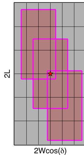
**Figure 1.** Seismic uncertainty rectangle and its associated faults. The red star denotes the estimated epicenter. The grey rectangle delimits the uncertainty area and it is centered at the epicenter, its dimensions being  $2L$  in length and  $2W\cos(\delta)$  wide, projected in the horizontal plane. The smaller pink rectangles indicate sample scenarios that include the epicenter. Grid in black denotes the unit sources domain.
