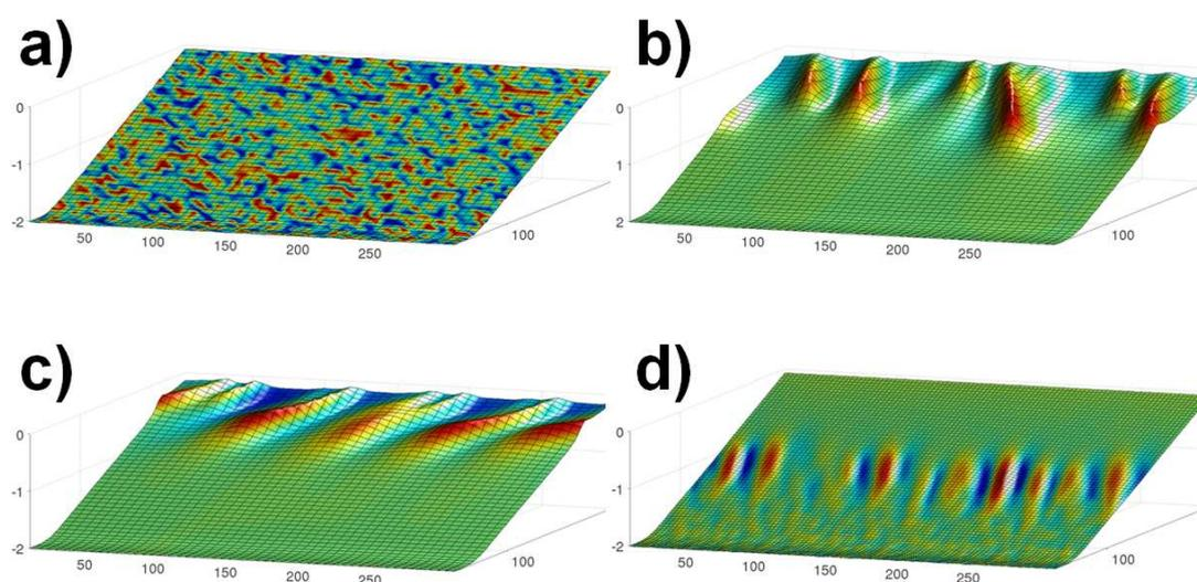
Figure 3. Three-dimensional view of the bed level. The colors represent the bed-level perturbations with respect to the mean profile (shoals are in red, troughs are in blue). (a) Initial bathymetry where random bed-level perturbations have been added. (b) Tidal forcing. (c) Wind forcing. (d) Wind-wave forcing. The experiments are performed by using a constant sediment stirring (Equation 8).
