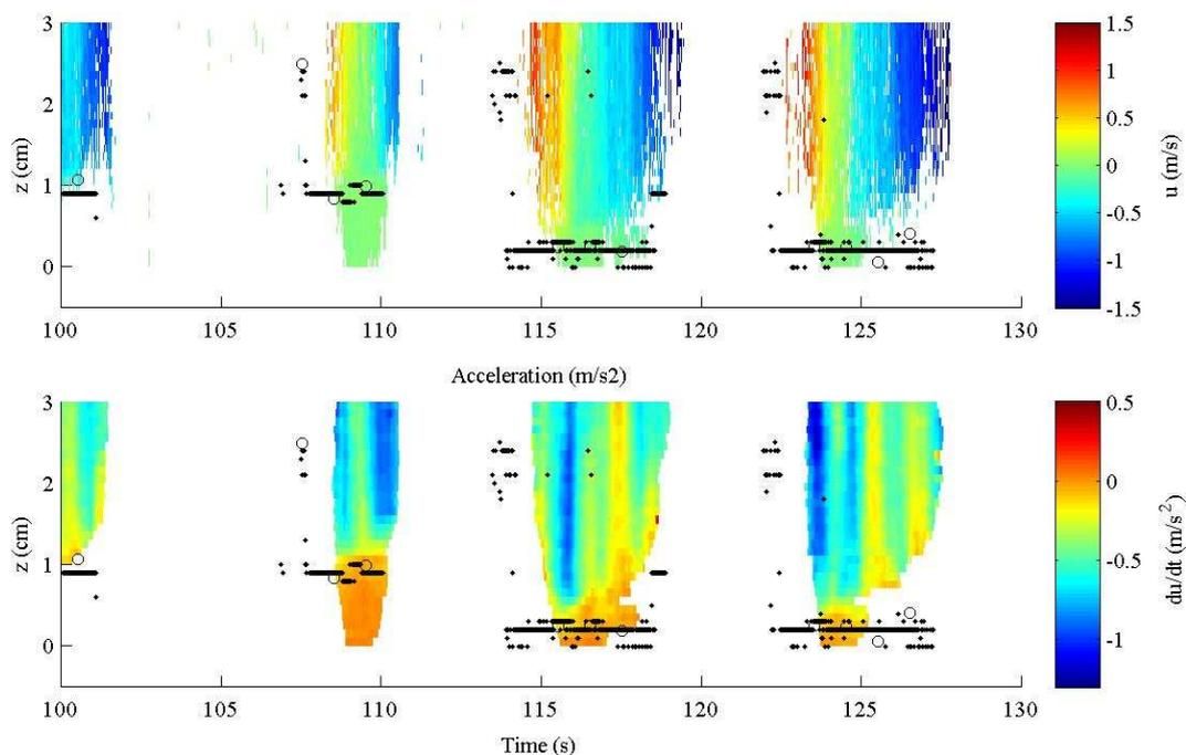
Figure 3. An example 30-second time series of (upper) horizontal velocity and (lower) local acceleration as a function of elevation.  $z=0$  represents the reference elevation. Onshore-directed flow is defined with positive velocities. The open circles represent the Vectrino II estimates of the bed elevation and the black dots represent the instantaneous bed elevations.
