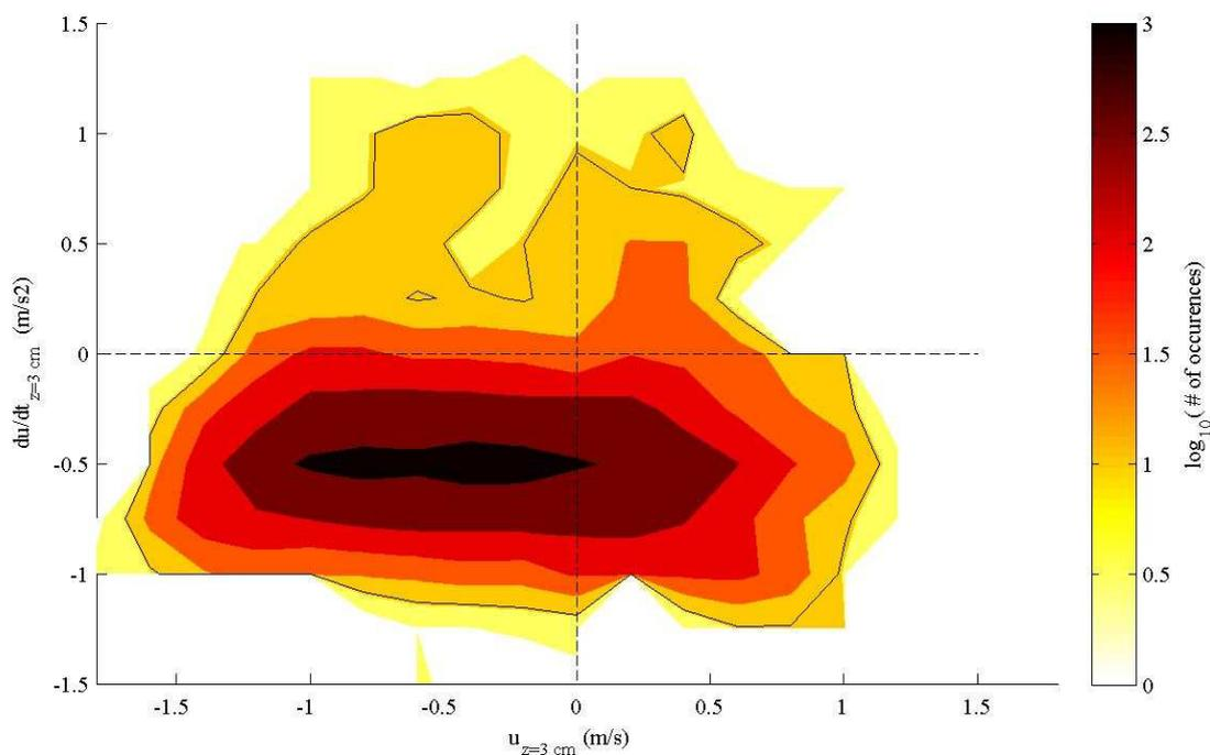
Figure 4. The phase space average distribution of the number of occurrences with each horizontal velocity and acceleration bin over a 10-minute realization. The colors indicate the  $\log_{10}$  of the number of occurrences.
