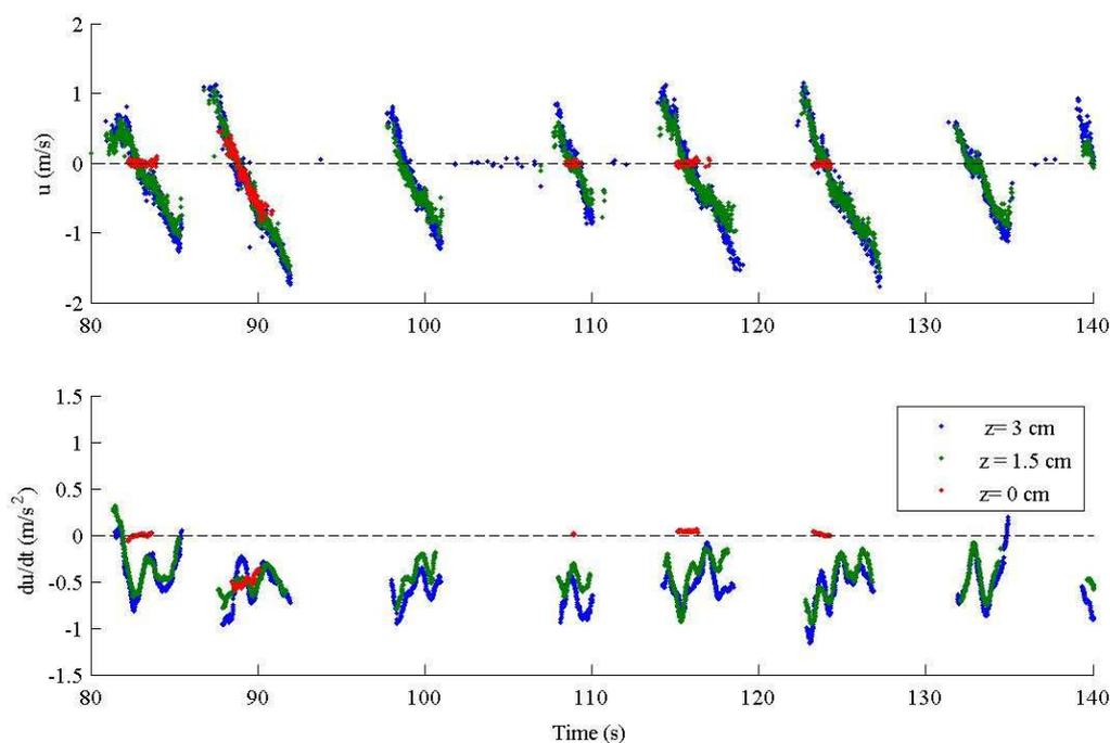
the SNR method described above are generally coincident with locations where the velocity and acceleration approaches zero.
