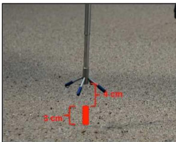
Figure 1. A snapshot of the Vectrino II over a dry sediment bed. The 3 cm profiling range is located below the 4 cm blanking distance.
