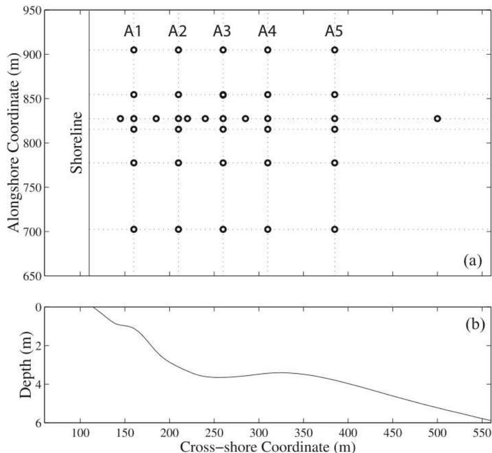
**Figure 5:** (a) Plan view of SandyDuck instrument array. Each circle indicates a velocity sensor. The Field Research Facility coordinate system is used where  $(x, y)$  are cross- and alongshore, respectively. The five alongshore arrays are indicated A1–A5. The approximate location of the shoreline is shown near  $x = 110$  m. (b) Alongshore-averaged depth below mean sea level versus cross-shore coordinate.
