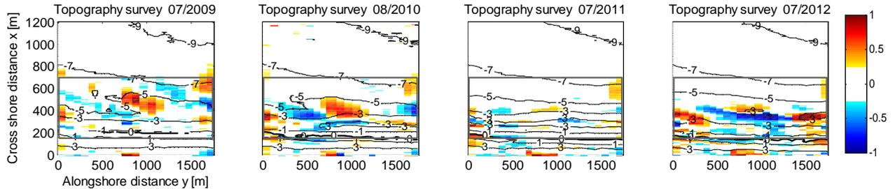
Figure 4. Planform images of alongshore variability  $z_{\text{var}}$  at Vlugtenburg beach in the summers of 2009 to 2012. Colors indicate the deviation  $z_{\text{var}}$  from the mean alongshore topography in meters. Contour levels indicate the bed level in m as displayed in Figure 2.
