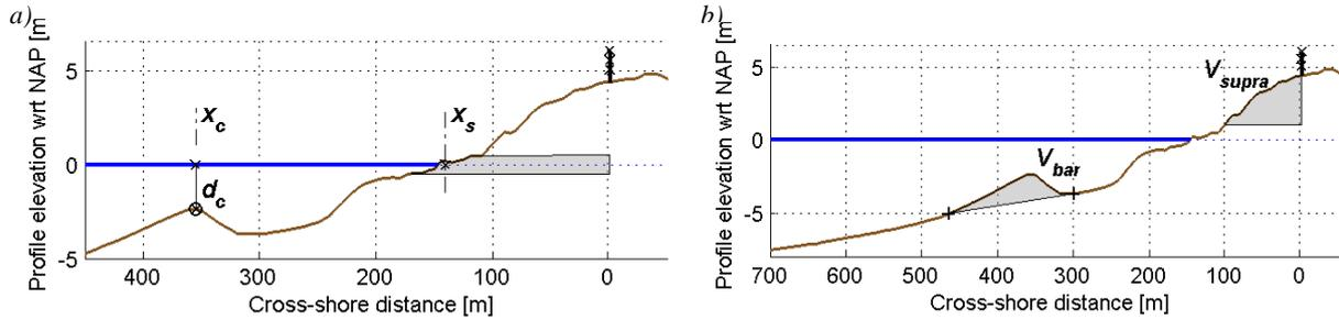
Figure 6. Profile parameters. a) Methodology to determine shoreline position  $x_s$ , bar crest location  $x_c$  and bar crest depth  $d_c$ , and b) Methodology to determine the volume of the supra tidal beach  $V_{supra}$  and the volume of the subtidal bar  $V_{bar}$ .
