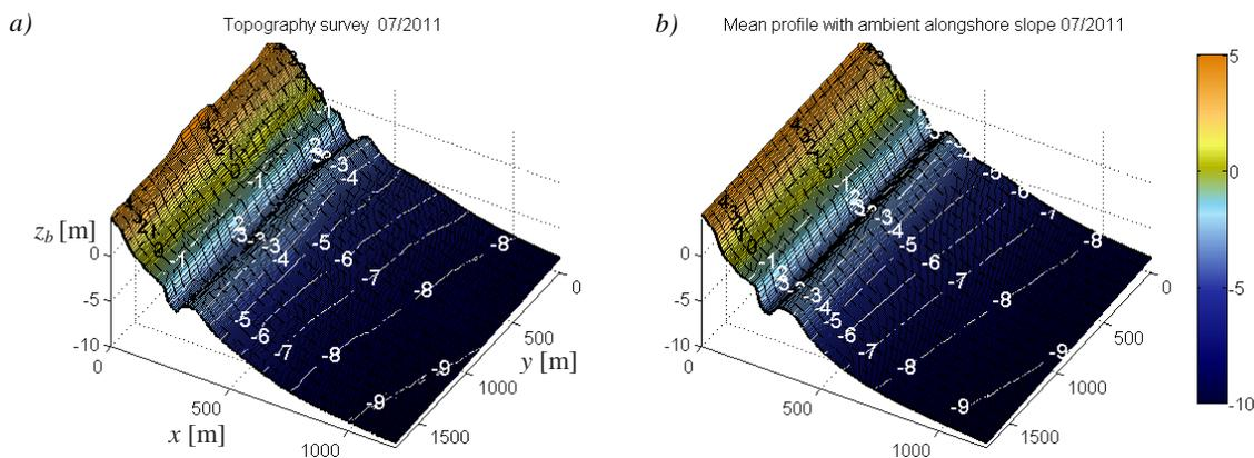
Figure 3. a) Interpolated survey profiles ( $z_b$ ) and b) alongshore averaged profile ( $z_{b,mean}^*$  Eq. 2) for June 2011. Note the angle of the deeper isobaths (-6 to -9 m) with respect to the shoreline.
