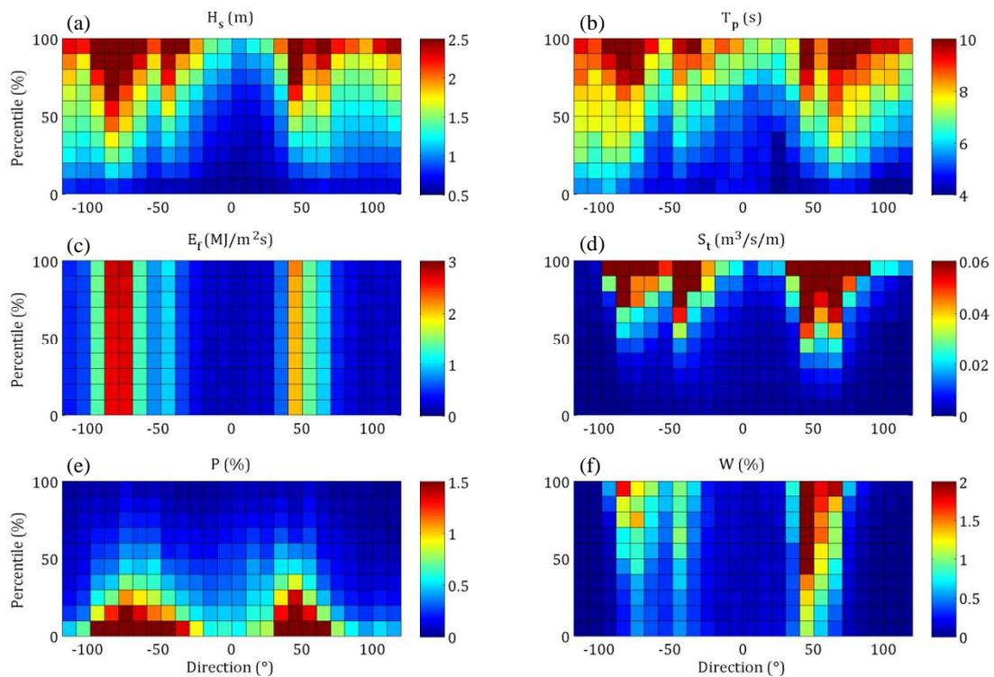
Figure 4 The discretized (high resolution) wave climate for Method 2. Within each cell is shown (a)  $H_s$ , (b)  $T_p$ , (c)  $E_f$ , (d)  $S_t$ , (e)  $P$  and (f)  $W$ . The color scale is indicated at the right of each plot and units shown in the title. The x- and y-axes are discretized in 24 directional sectors and 10 percentile classes of  $E_f$ , respectively
