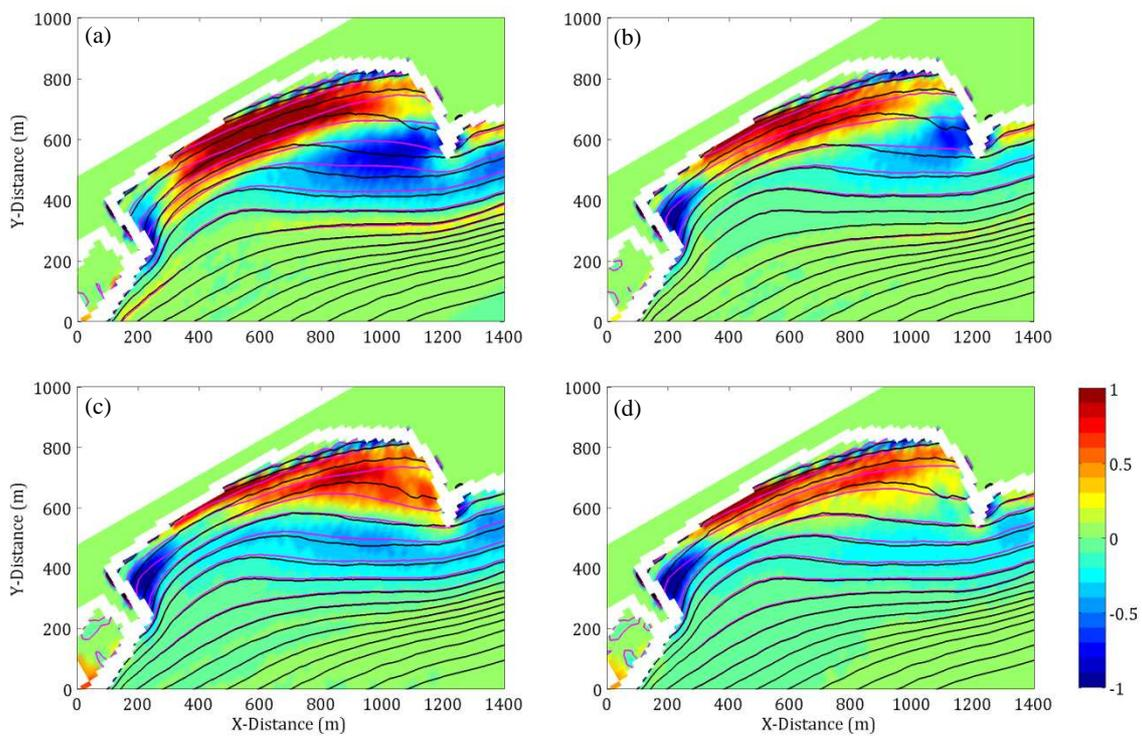
Figure 9 Difference (color scale) between  $z_{eq,meas}$  (black contours) and  $z_{eq,rwc}$  (pink contours) where  $N_{rwc} =$  (a) 4, (b) 8, (c) 12, and (d) 16, for Method 2. Contours are drawn every 1.5 m between +1.5 m and -24 m
