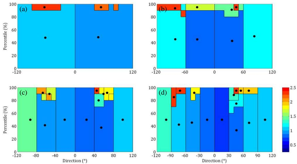
Figure 6 Clustering of RWC bins for (a) 4 bins, (b) 8 bins, (c) 12 bins, and (c) 16 bins for Method 1. The color scale and the position of the black dots relative to the x-axis indicates the value of  $H_{s,rwc}$  and  $\theta_{rwc}$ , respectively
