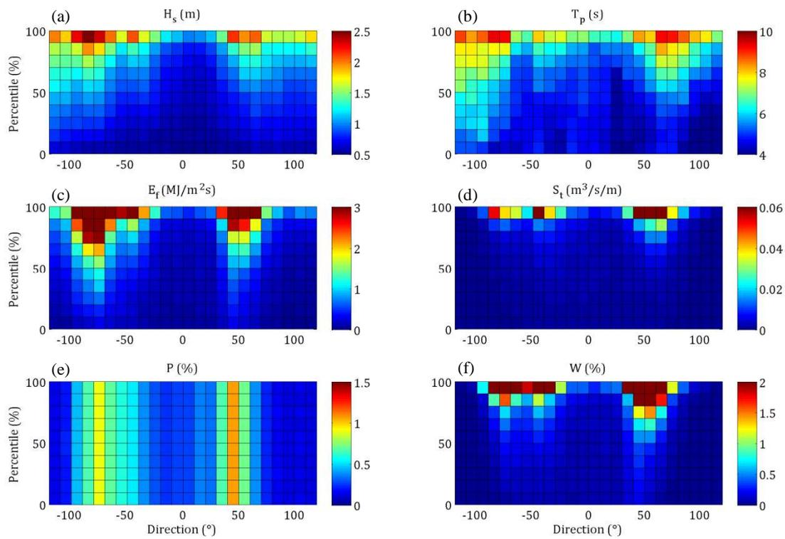
Figure 3 The discretized (high resolution) wave climate for Method 1. Within each cell is shown (a)  $H_s$ , (b)  $T_p$ , (c)  $E_f$ , (d)  $S_t$ , (e)  $P$  and (f)  $W$ . The color scale is indicated at the right of each plot and units shown in the title. The x- and y-axes are discretized in 24 directional sectors and 10 percentile classes of  $P$ , respectively
