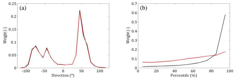
Figure 5 Weighting factor,  $W_{dwc}$  plotted over the (a) wave direction and (b) percentiles of  $P$  (for Method 1, black line) and percentiles of  $E_f$  (for Method 2, red line)
