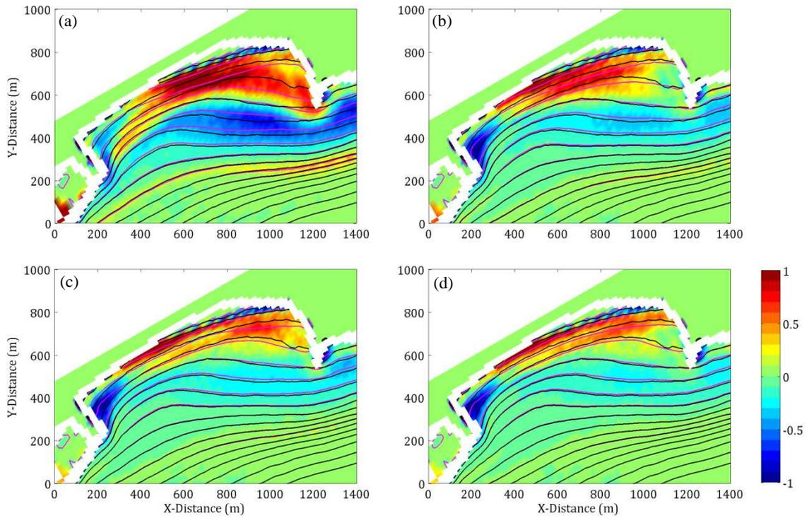
Figure 8 Difference (color scale) between  $z_{eq,meas}$  (black contours) and  $z_{eq,rwc}$  (pink contours) where  $N_{rwc} =$  (a) 4, (b) 8, (c) 12, and (d) 16, for Method 1. Contours are drawn every 1.5 m between +1.5 m and -24 m
