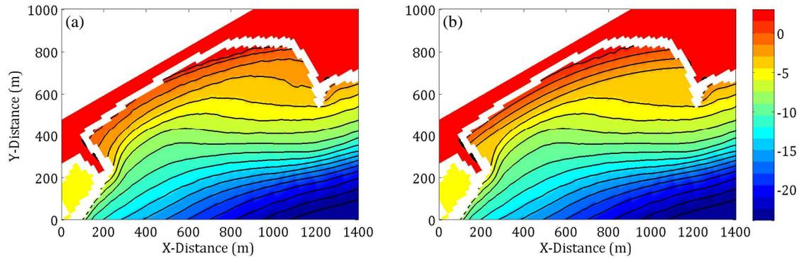
Figure 2 (a) Average of measured bathymetries of the bay,  $z_{eq,meas}$ . (b) Initial bathymetry used for morphodynamic simulations,  $z_{ini}$ . Contours are drawn every 1.5 m between +1.5 m and -24 m
