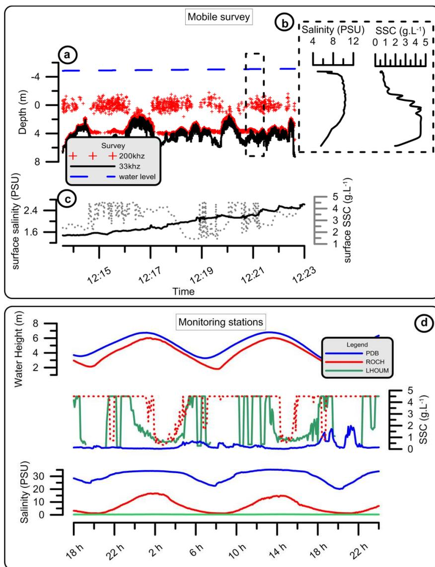
Figure 2: Survey data and associated turbidity probe, time-series of monitoring station, 12 October 2012.
