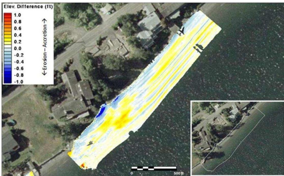
Figure 10. Elevation difference at Point White – Site 4 between 12 November and 11 December 2012.
