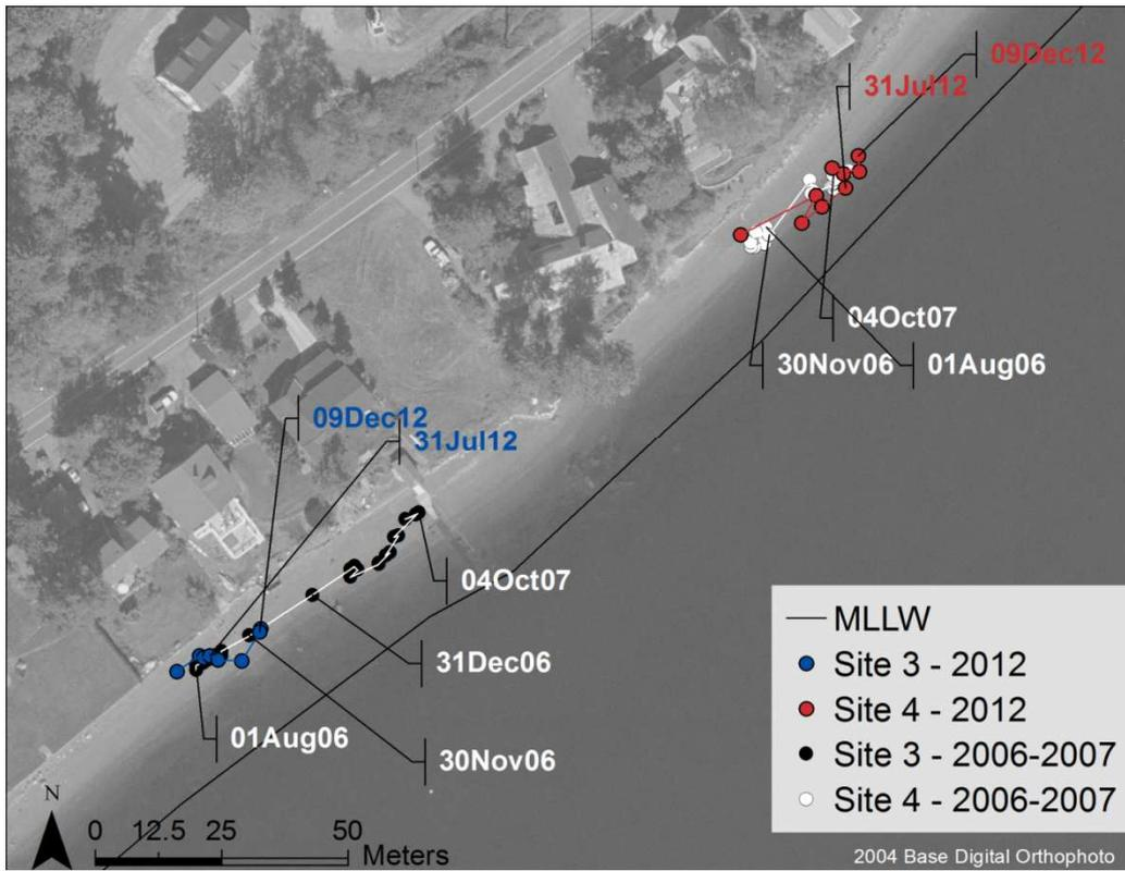
Figure 7. Location of tracer centroids for the 2006-2007 and 2012 survey at Sites 3 and 4
