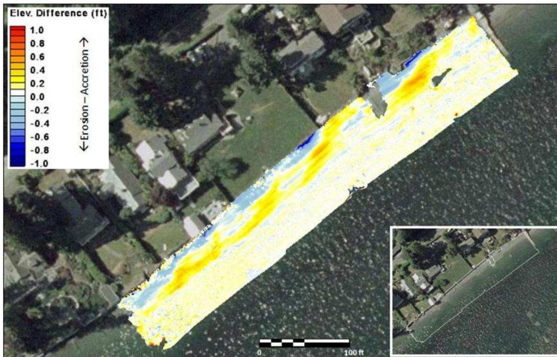
Figure 8. Elevation difference at Point White – Site 3 between 12 November 2012 and 11 December 2012
