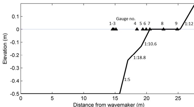
Figure 1: Laboratory setup for the University of Michigan flume experiment (Demirbilek et al., 2007).
