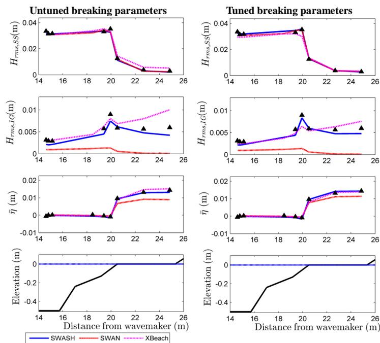
Figure 2. Measured (black triangles), and simulated  $H_{rms,SS}$ ,  $H_{rms,IG}$  and  $\bar{\eta}$  across the UM fringing reef profile for Test no. 35 ( $H_{rms,SS}=0.032$  m;  $T_p=1.42$ ;  $h_r=0.00$  m). Model results for untuned (left column) and tuned (right column) breaking parameters are shown for SWASH (solid blue curve), SWAN (dotted red curve), and XBeach (dashed magenta curve). The reef elevation profile is shown in the bottom row for reference.
