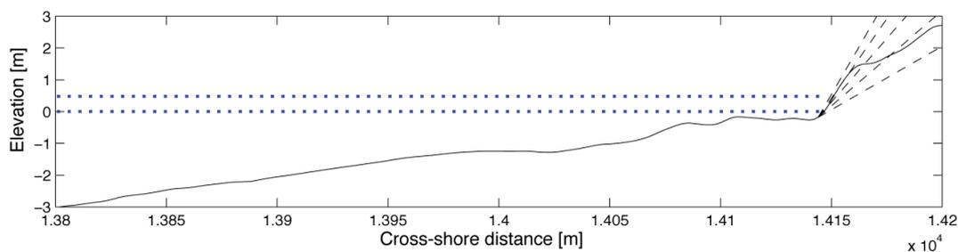
Figure 4. Beach profiles used to estimate the influence of the foreshore slope on run-up statistics at Tizimin. The solid line is the measured beach profile, whereas the dashed lines represent the different foreshore slopes (0.04, 0.06, 0.08, 0.1 and 0.12) employed in the simulations. The dotted lines represent the mean and high-tidal level (+0.5 m).
