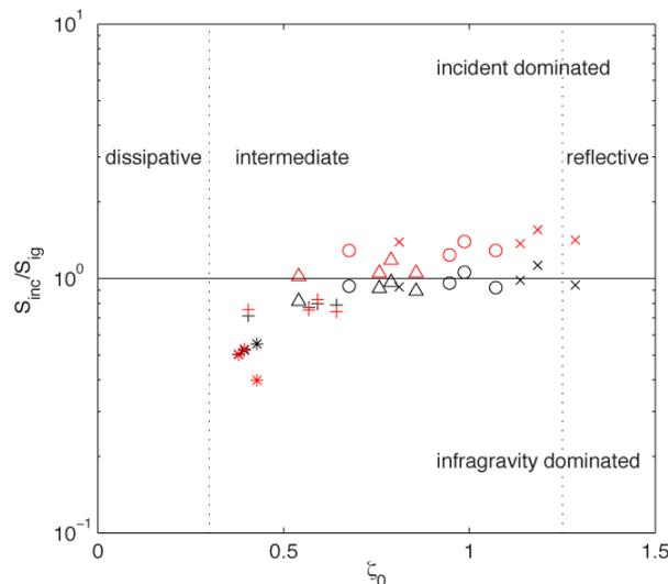
Figure 6. The ratio  $S_{inc}/S_{ig}$  versus  $\zeta_0$ , for (black) mean water level and (red) high-tide level. Symbols denote the foreshore slopes (\*) 0.04, (+) 0.06, ( $\Delta$ ) 0.08, ( $\circ$ ) 0.10 and ( $\times$ ) 0.12. Conditions with  $\zeta_0 < 0.3$  are determined as dissipative,  $0.3 < \zeta_0 < 1.25$  as intermediate and  $\zeta_0 > 1.25$  as reflective.
