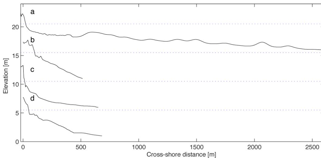
Figure 2 - Measured bottom profiles at (a) Dzilam, (b) Hunucma, (c) Progreso and (d) Tizimin to 4 m depth, used in the SWASH model simulations. The profiles are vertically spaced with 5m difference, dotted lines represent the mean water level at high tide conditions (+0.5 m).
