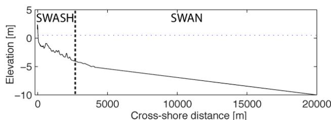
Figure 3. The simulations were performed between 10 – 4 m depth with the SWAN model, for the section from 4m till shore with the SWASH model. The Dzilam profile is used for illustration, the horizontal dotted line is the mean high tide level and the vertical dashed line represents the transition between the SWAN and SWASH simulations.
