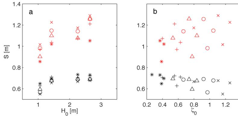
Figure 5. Predicted swash height ( $S$ ) versus (a) deep water wave-height  $H_0$  and (b) Iribarren number  $\zeta_0$  for the simulations with a variable foreshore slope. Black symbols represent simulations with mean water level and red symbols those with the high-tide level. Foreshore slopes were (\*) 0.04, (+) 0.06, ( $\Delta$ ) 0.08, ( $\circ$ ) 0.10 and ( $\times$ ) 0.12.
