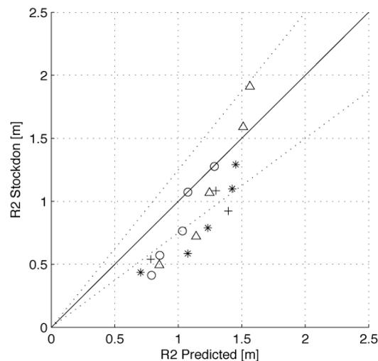
Figure 9. Parameterization of the 2% exceedence value by Stockdon et al. (2006) for the run-up simulations versus the predictions. The solid line represents the line of equality, dotted lines a 25% difference.
