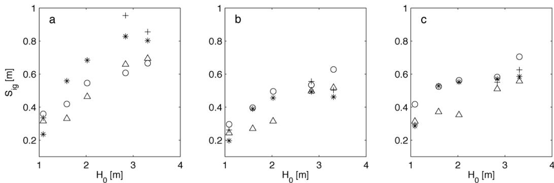
Figure 8. Infragravity swash height  $S_{ig}$  versus offshore wave height  $H_0$  for (a)  $0.004 < f < 0.025$ , (b)  $0.025 < f < 0.035$  and (c)  $0.035 < f < 0.05$ Hz. With (\*) Dzilam, (O) Hunucma, (Δ) Progreso and (+) Tizimin.
