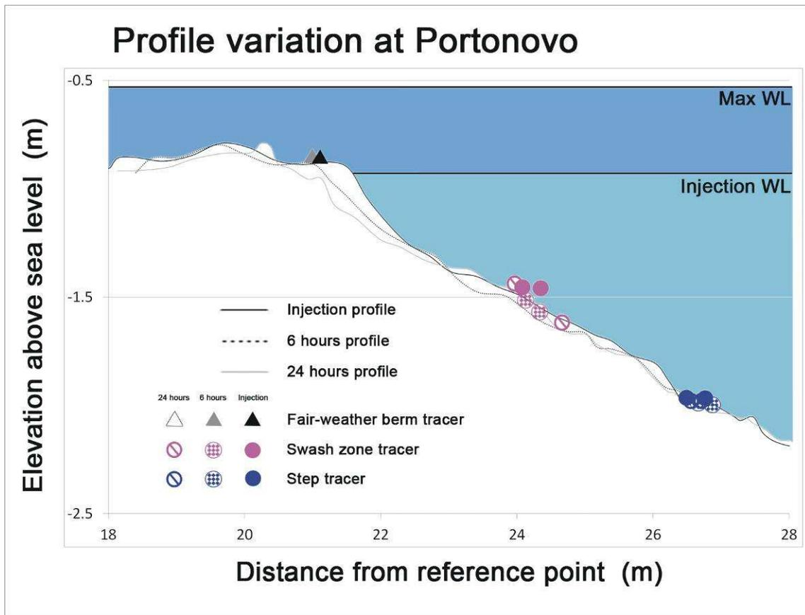
Figure 5. The evolution of the reference profile during the time frame of the experiment
