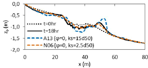
Figure 6. Experimental results (dotted and solid lines) and computed (dashed lines) profiles of 18h simulation, using the formulations of N06 and A13. The computed profiles consider the bed shear stress predictor with  $\phi = 0^\circ$  and  $k_s = 2.5d_{50}$  or  $k_s = 15d_{50}$ , respectively.
