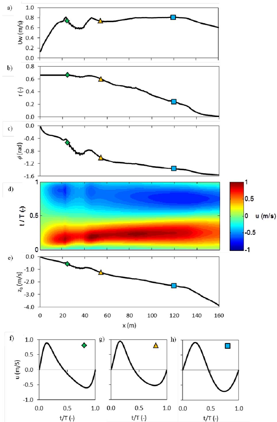
Figure 3. (a) Linear wave, near-bed, orbital velocity  $U_w$ , (b) non-linearity parameter  $r$ , (c) waveform parameter,  $\phi$ , (d) horizontal velocity  $u(t)$  and (e) bed elevation  $z_b$  versus cross-shore distance  $x$ . Panels (f), (g) and (h) show the temporal variation of  $u(t)$  for three cross-shore positions indicated with symbols (diamond –  $x=24.5$  m; triangle –  $x= 54.5$  m; rectangle –  $x= 119.5$  m).
