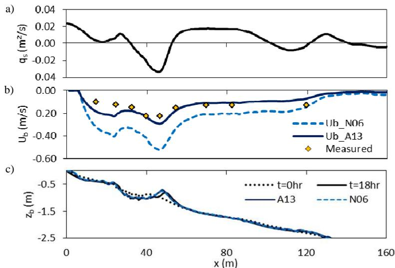
Figure 7. (a) Measured sand transport,  $q_s$ , from bed level soundings at  $t=0$  and  $t=18$  hr; (b) Measured (diamonds) and computed values of the undertow that lead to the values of  $q_s$  using the formulations of N06 (dashed line) and A13 (solid line).
