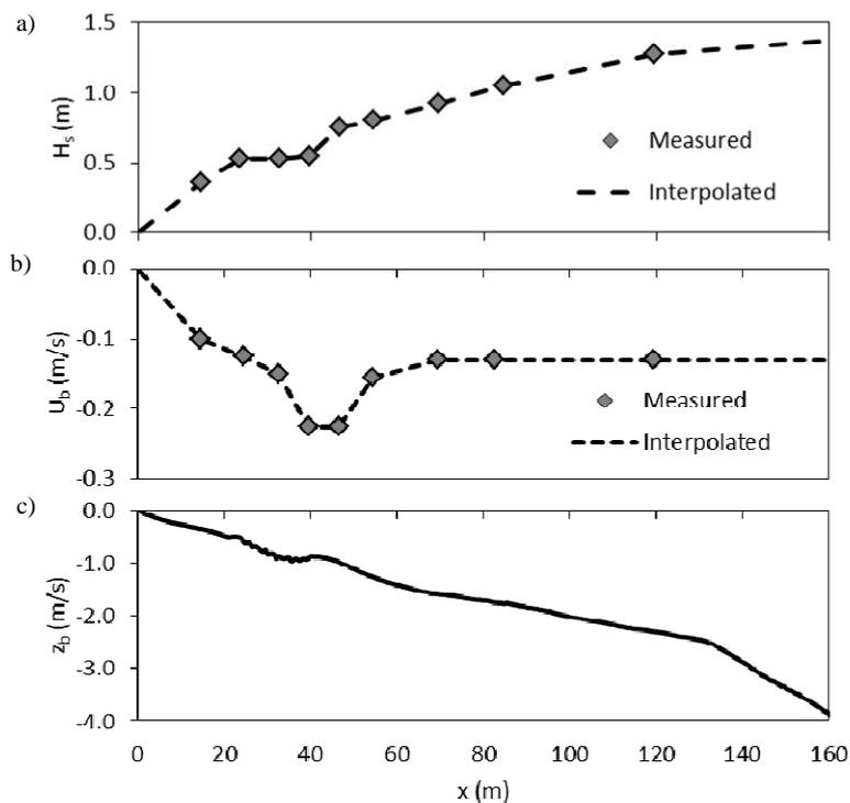
Figure 1. (a) Significant wave height  $H_s$ , (b) undertow and (c) bed elevation  $z_b$  versus cross-shore distance  $x$ . Diamonds indicate measured values whereas the dotted lines correspond to linear interpolations between these values.
